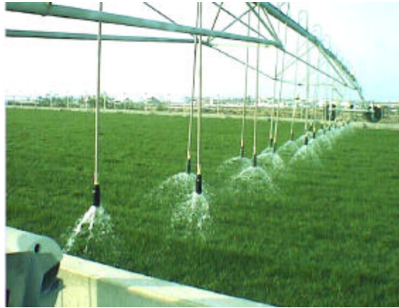
Figure 3.13. Feeding an infiltration percolation unit in Torre Vieja (Spain)
