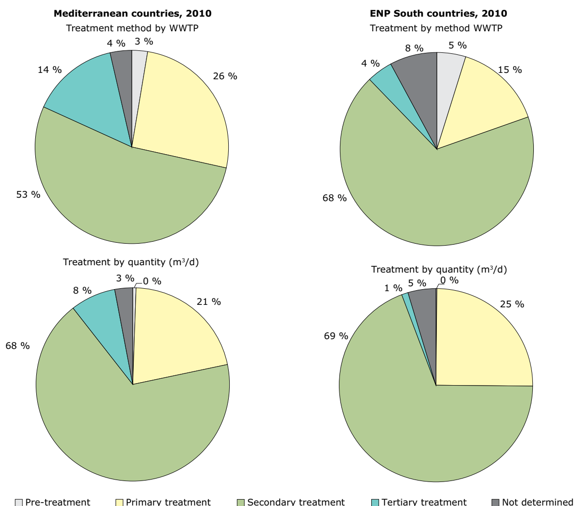
Figure 4.12 Distribution of treatment method by WWTP and by wastewater quantity for Mediterranean countries and ENP-South countries
