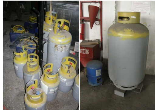
Figure 26: Smaller cylinders and equipment (blue) used for ODS recovery and storage (left) with unused large tank (right). Polair, Kazakhstan.
