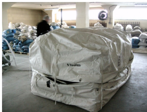
Figure 37: Cocoon for creating low oxygen environment to kill pests on seeds. PNOS Seed Company, Poland.
