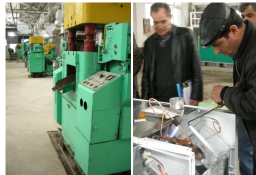
Figure 53: Template unit for cutting out door lining (left), welding compressor circuit to compressor (right), and finished refrigerators (below). SINO, Uzbekistan.
