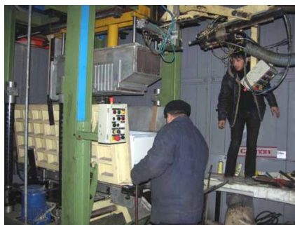
Figure 14 Cannon cabinet foaming jigs
