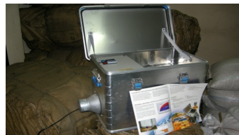
Figure 19: Speedbox for rapidly releasing phosphine pesticide into flour mills. Yandi Company, Bulgaria
