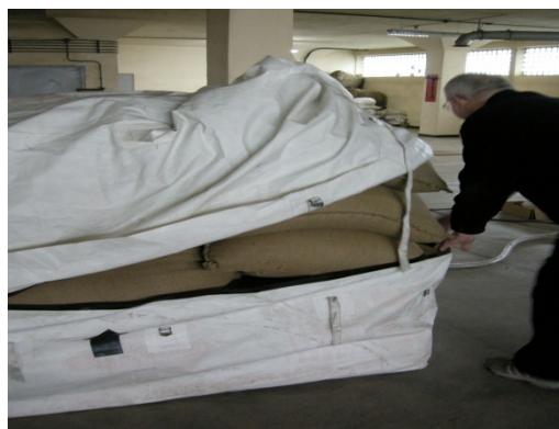
Figure 38: Cocoon for creating low oxygen environment to kill pests on seeds, with damaged zipper. PNOS Seed Company, Poland.
