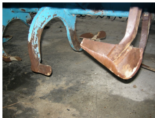
Figure 36: Spader showing nematocide bins (red), and details of spades that are damaged by rocks in soil. Solfum, Poland.
