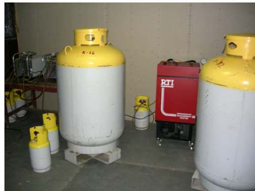
Figure 50: ODS reclamation equipment and storage cylinders (above), and recovery equipment (below). Shark Shaboda, Uzbekistan.
