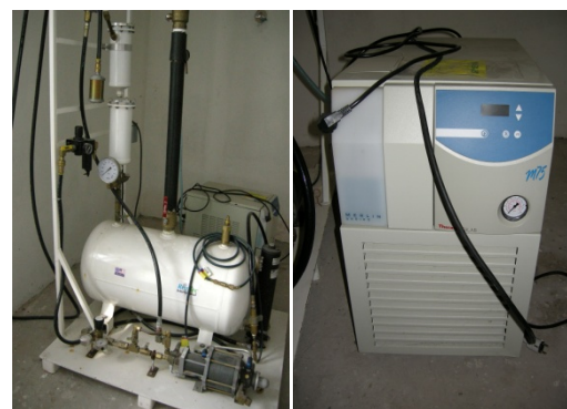
Figure 29: Little-used halon recovery and reclamation equipment. Polygon Research Centre, Kazakhstan
