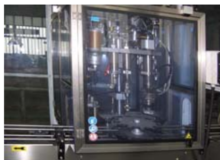
Figure 11: Coster gassing and crimping unit at YHCP
