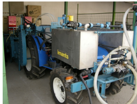
Figure 23: Rotary spader adapted for use in glasshouses with nematocide as liquid (front tanks) or granules (red rear tanks). Zephyr, Hungary.
