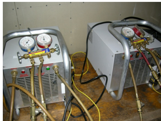
Figure 50: ODS reclamation equipment and storage cylinders (above), and recovery equipment (below). Shark Shaboda, Uzbekistan.
