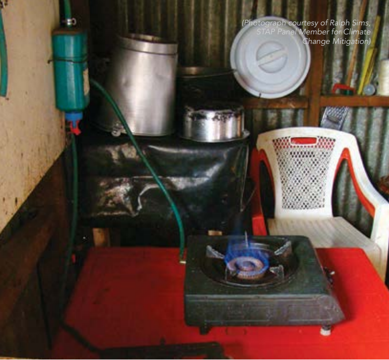
Clean burning biogas-fueled stove in the dwelling of a 4 cow dairy farmer in Kenya, that reduces black carbon emissions and improves health by replacing woody biomass combustion for cooking and milk pasteurization.
