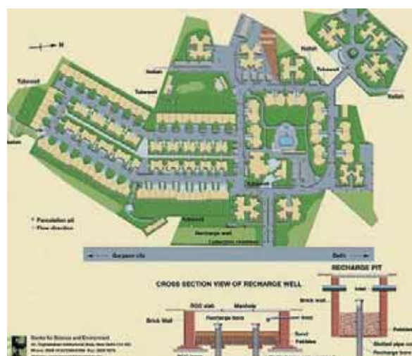
Illustration 53: Surya Vihar Rainwater Harvesting Systems, isometric view and cross sections percolation pit and recharge trench (top), Nizamuddin East Colony's Rainwater Harvesting Systems, site plan and cross section recharge well (middle), Garden Estate Rainwater Harvesting System, site plan and cross sections of rainwater harvesting well and recharge pit (bottom).
