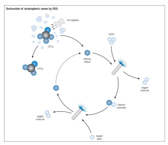
How ozone is destroyed after ultraviolet radiation liberates a chlorine radical from an ozonedepleting substance. One chlorine atom alone can take part in as many as 100 000 ozone-destroying reactions.
