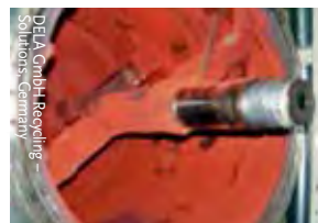
Vacuum mixer to form solid mercury sulphide
