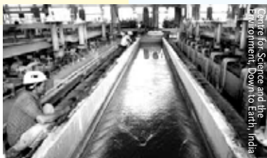
An open mercury-cell at a chlor-alkali plant.
