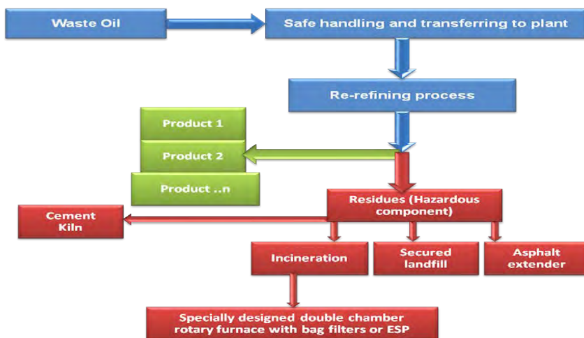
Figure 2.3.1: General schematic of the waste oil recycling process
