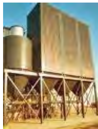
Picture 2.16.1.5.3 A typical bag house filter
