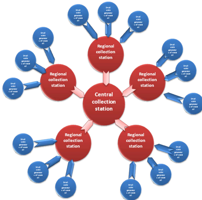
Figure 1.8.2.2.b: Multi-layered collection system for waste oils
