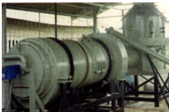
Picture 2.16.1.4 A typical rotary kiln incinerator
