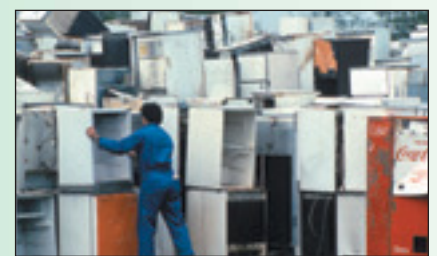
CFC-laden foam must be removed from millions of discarded refrigerators in the UK
