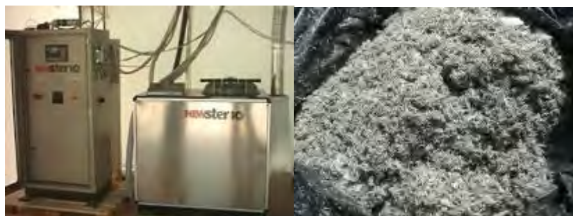
Figure 11.27. Newster 10 (L) and close-up of treated waste (R); similar to the unit installed in Bolak El Dakroor Hospital, Egypt
