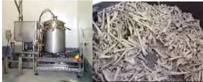
Figure 11.29. WR 2 alkaline hydrolysis unit and close-up of bone residues; similar to the unit installed at the Backweston Veterinary Lab, Ireland
