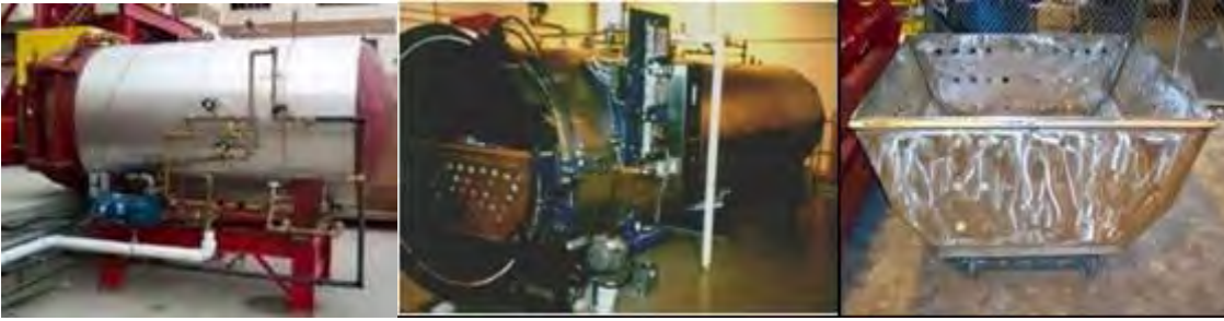
L-R: Moss autoclave (side view), autoclave with a waste cart inside, stainless steel waste cart
