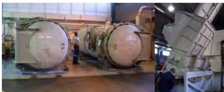
Figure 11.19. Large vacuum autoclaves (L) and shredder (R) at the Compass plant in South Africa
