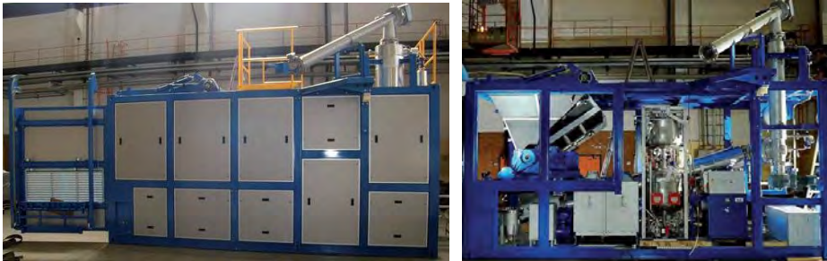
L-R: LogMed 400 closed, LogMed 400 with outer covering removed
