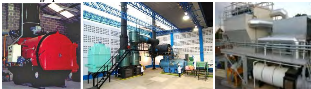
L-R: Techtrol Pyrotec clinical incinerator, Incol incinerator with scrubber, Incol heat recovery boiler and catalytic gas cleaning system
