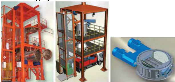
L-R: Pre-shredding L type, Pre-shredding V type, cassette-type shredder
