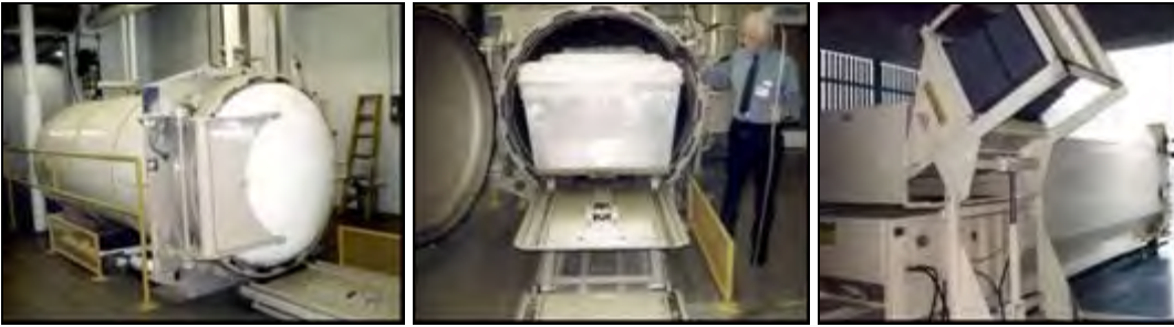
L-R: Bondtech autoclave, on-site autoclave with lift table at a hospital, waste dumper
