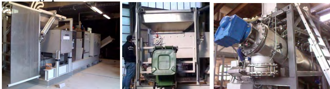
L-R: Log 100, hopper-shredder section, motor and isolation valve at the end of the auger
