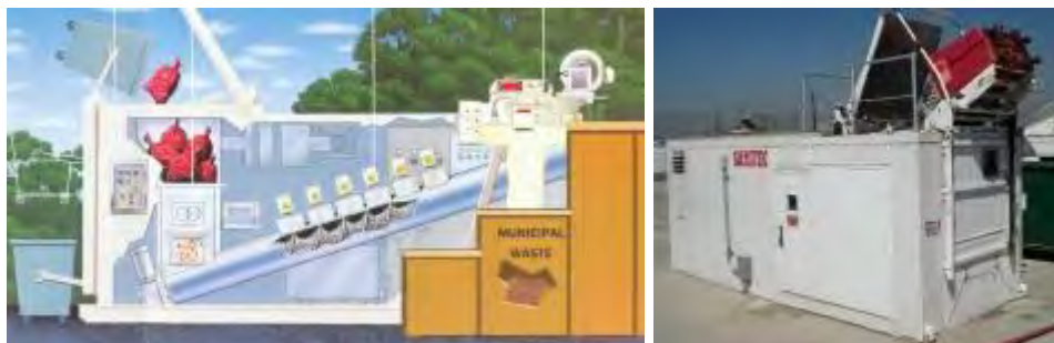
Figure 11.26. Sanitec microwave cut-out sketch and photo similar to the unit in CESI, Philippines
