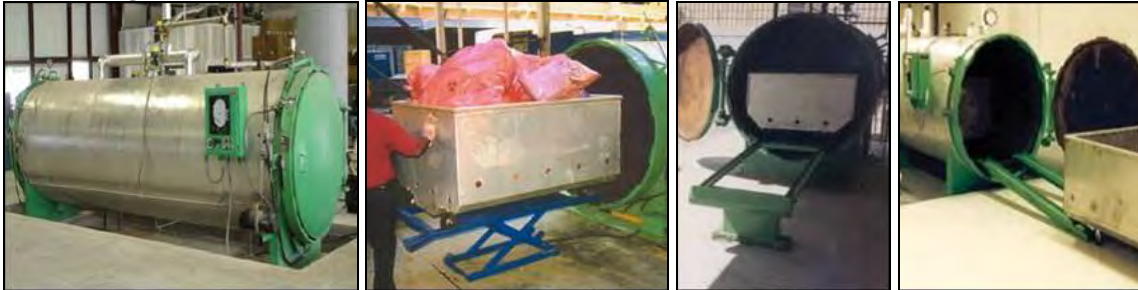
L-R: Mark-Costello autoclave (side view), waste cart being loaded in the AS58 autoclave via a hydraulic lift, AS 58 autoclave with a pull-out drawer for waste, autoclave with a cart ramp
