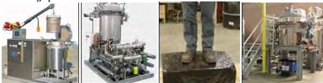
L-R: Caustic Digester Unit (CDU) with 36 kg capacity, CDU with 300 kg capacity, solidified mass from the CDU, Thermal Tissue Digester (TDU) 500
