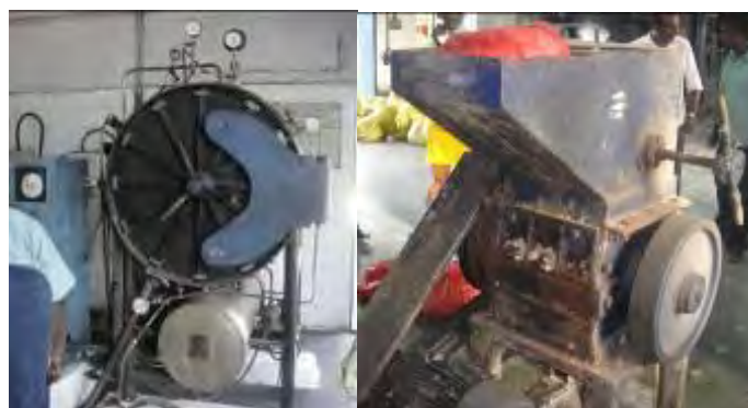
Figure 11.18. Autoclave (L) and shredder (L) at the GJ Multiclave Central Treatment Facility, India
