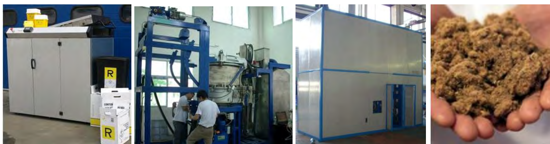
L-R: OMPeco Converter Models H10, H75, H200 and close-up of treated waste
