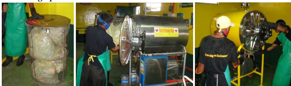
L-R: Waste in stainless steel wire basket; loading basket, starting the cycle
