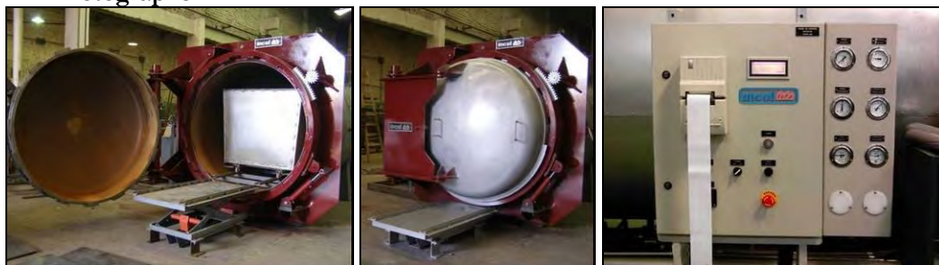
L-R: Incol autoclave showing lift table and cart, autoclave with door closed, control panel
