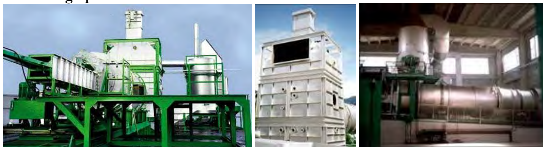
L-R: Hafner mobile rotary kiln incinerator, secondary chamber, stationary rotary kiln incinerator
