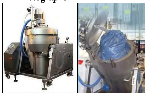
L-R: Ecolotec unit, close-up of sterilizing bowl tilted during loading
