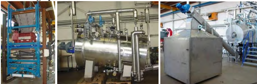
L-R: Lift and tilting mechanism with shredder and hopper, sterilization chamber, screw conveyor and discharge unit
