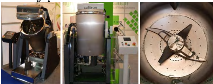
L-R: ISS unit in the tilted and vertical positions; close-up of the shredder blades
