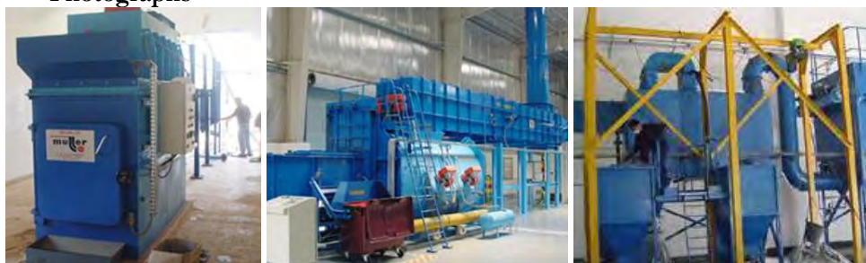
L-R: Models CP100, HP1000, neutralizing dry scrubber and filter
