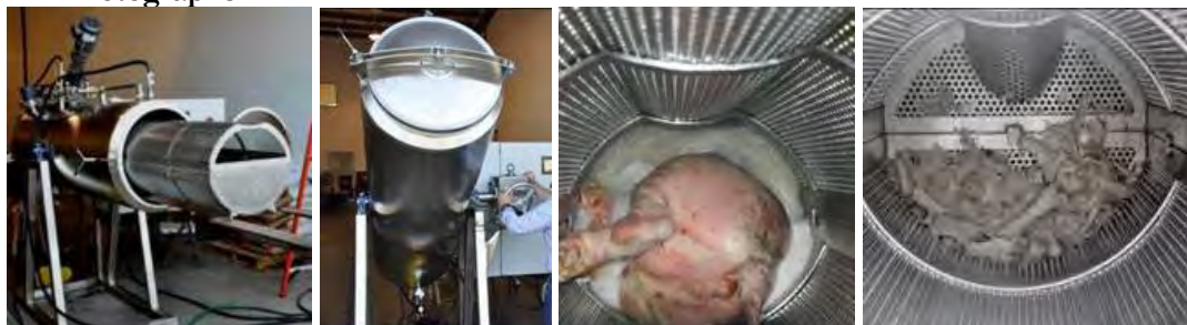
L-R: Low-temperature unit showing steel basket, unit being tipped up for operation, test pig carcasses before treatment, bone residues after treatment
