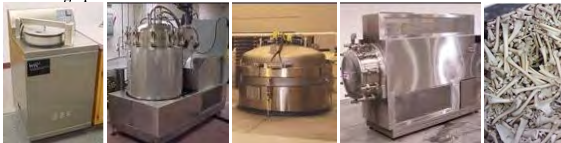
L-R: Tissue Digestors: low pressure small lab unit, medium capacity unit, large capacity unit, human cadaver unit; close-up of bone residues after treatment
