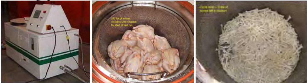
L-R: PWS D-2 unit, 66 kg of chicken before treatment, 3 kg of bones left after treatment
