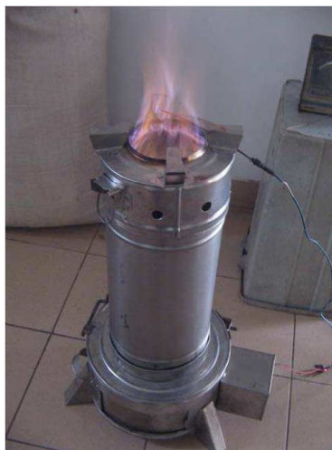
Figure 4: Low Cost Rice Husk Gasifier Stove
