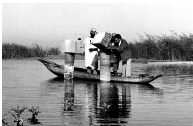
Figure 13 Measuring water levels at Kindjeria (centre of northern pool) in 1975. This gauge is presently not in operation. (Photo: Chouret in USGS 2001)
