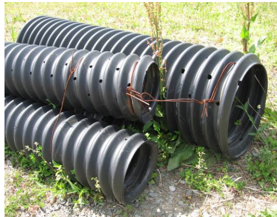
Photo- 17: Samples of Leachate Collection Pipe
