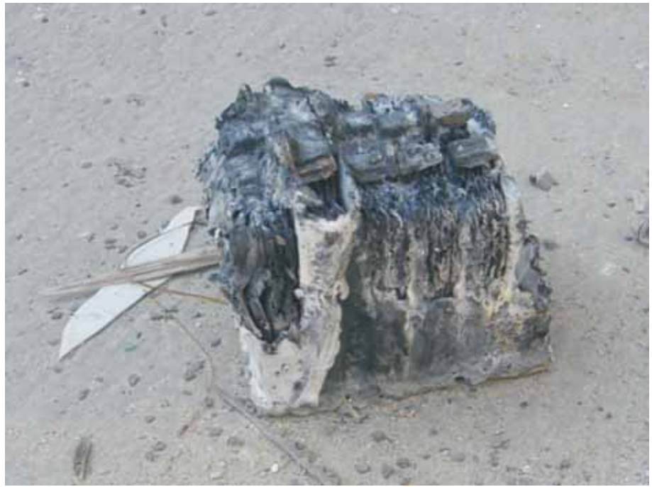
The remains of a burned lead-acid battery at Nieve Dkalim
