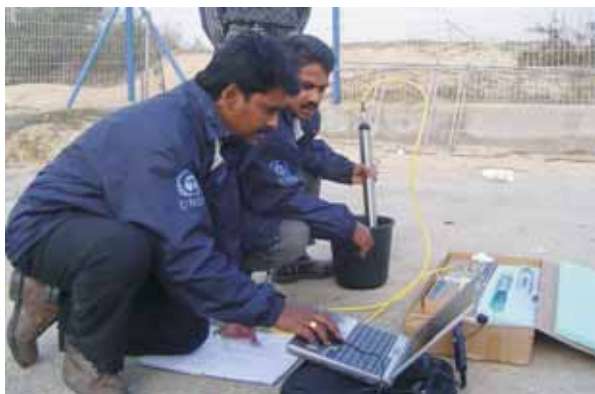
UNEP experts operating Multi Parameter Field Analyser
