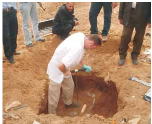
UNEP expert collecting a core sample from an excavation pit
