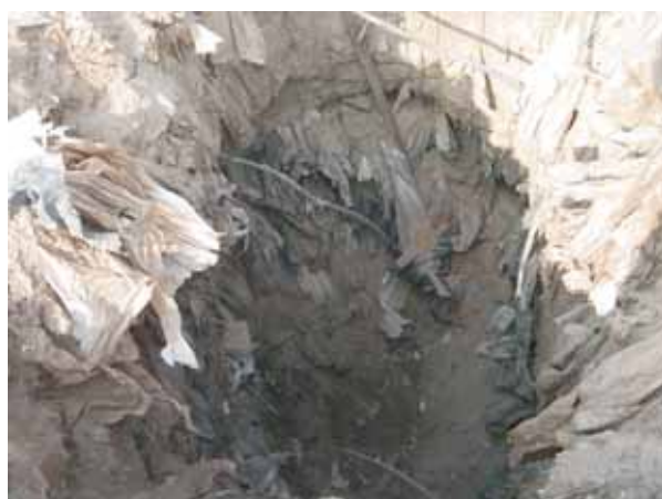
High volumes of plastic and organic material in an excavation pit
