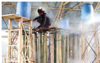
The current bamboo treatment system in operation – each bamboo is stacked vertically and filled with a treatment solution while being smoked
