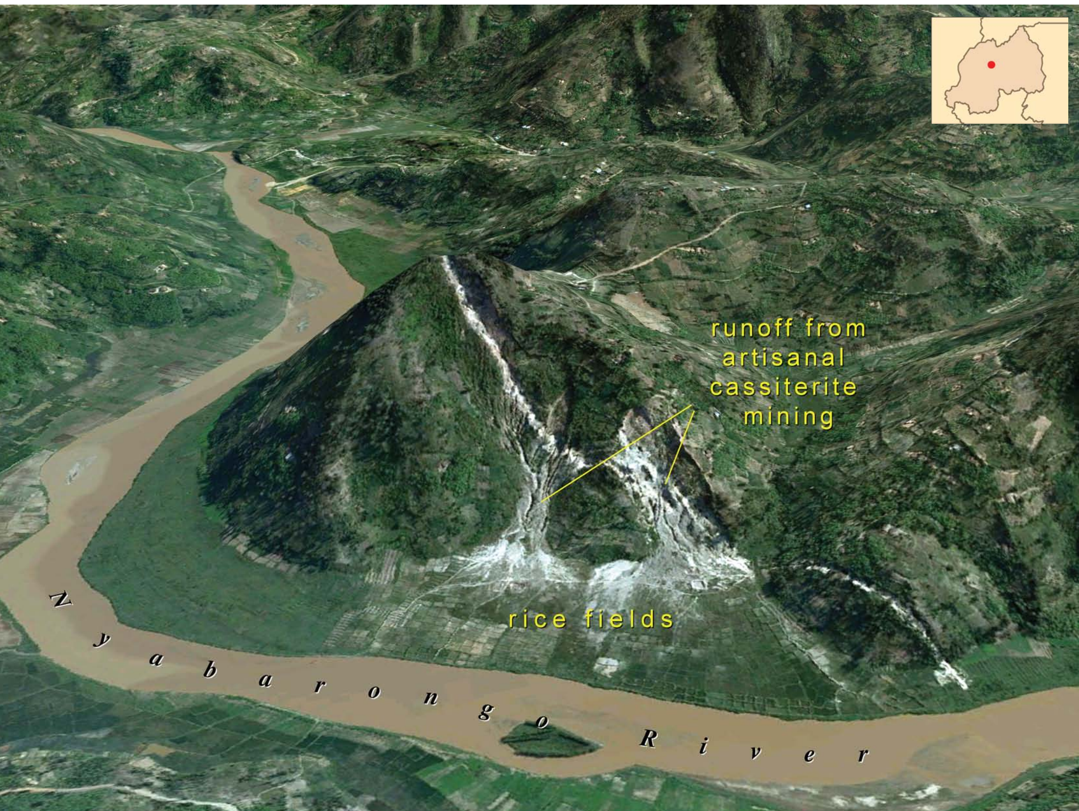
An orthophoto image showing cassiterite (tin ore) residues from open cast artisanal mining in Gakenke District flowing into rice paddies and into the Nyabarongo River.
