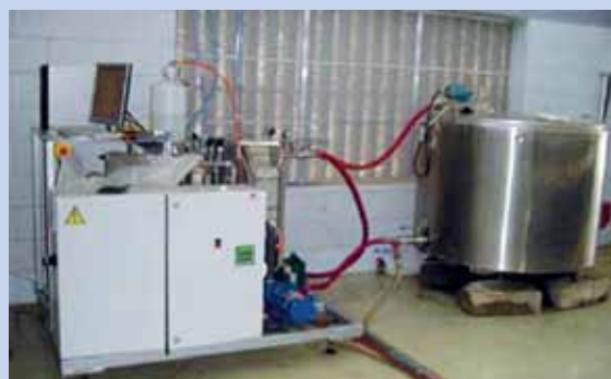
FIGURE B3 PHOTOGRAPHS OF MD PILOT PLANT
