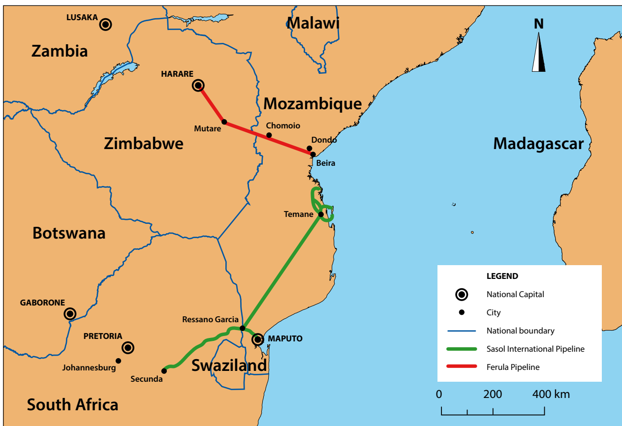
Figure 26.3. The Sasol Natural Gas project map, showing pipeline extending from the coastal gas fields of Temane and Pande to the industrial hub at Secunda in South Africa. Note: the Feruka pipeline, built in 1966, is 408 km long and supplies fuel oil to Harare, Zimbabwe. A similar pipeline exists in Tanzania, the Tazama pipeline, commissioned in 1968, extending 1 710 km from Dar es Salaam, supplying oil to Ndola, Zambia. Modified from: Wildcat International FZ-LLC 2013.
