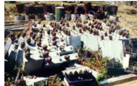
Picture 84: Bad example I (open air storage)
