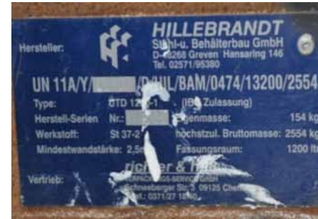
Picture 63: Example of UN approval plate
