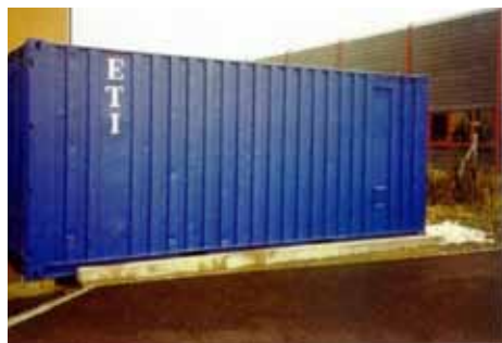
Picture 88: Typical 20' Box Container with drip tray
