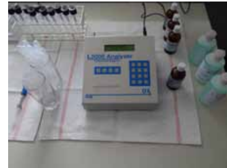
Picture 27: L2000 PCB / Chloride Analyzer
