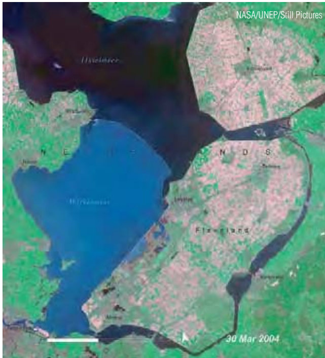
ZUIDERZEE WORKS, HOLLAND. The Zuiderzee Works are a man-made system of dams, land reclamation and water drainage works, and the largest hydraulic engineering undertaken by the Netherlands during the twentieth century.
