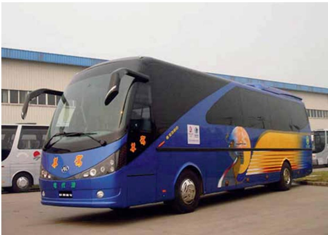
A prototype battery-supercapacitor all-electric bus
