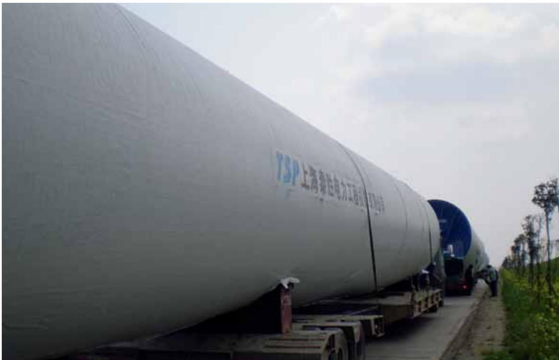
Part of the giant steel tower for a 1.5 MW turbine carried to the site to be erected in the Laogang Landfill.
