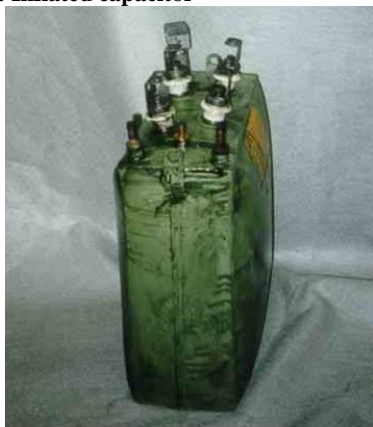
Picture 42: Inflated capacitor
