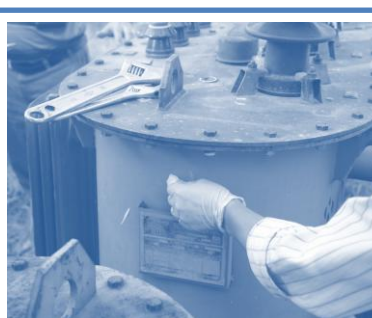
Affix sampling label on transformer (after cleaning the surface)
