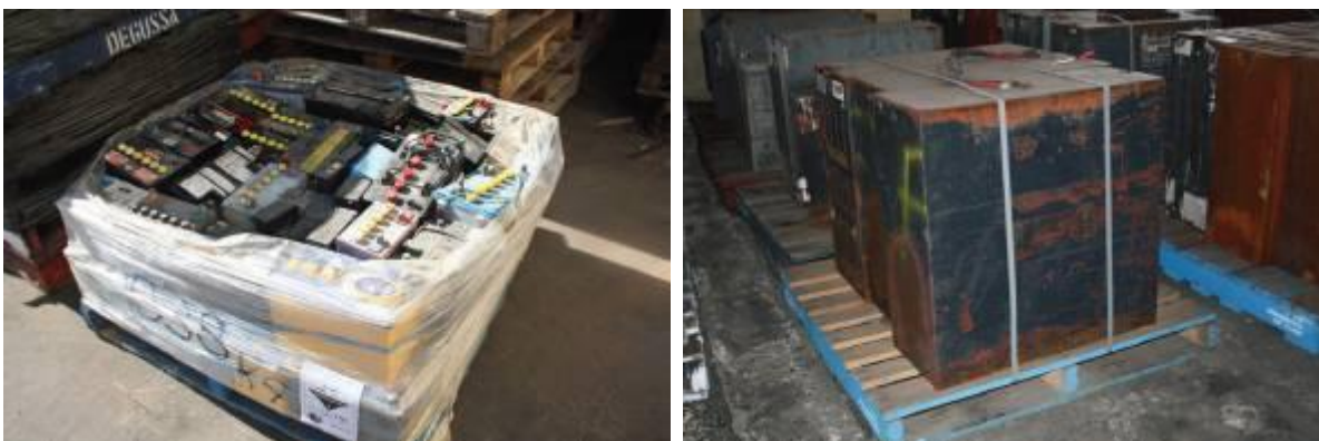
Fig. 40: Examples of bad packaging before transport, ABRI [26].
