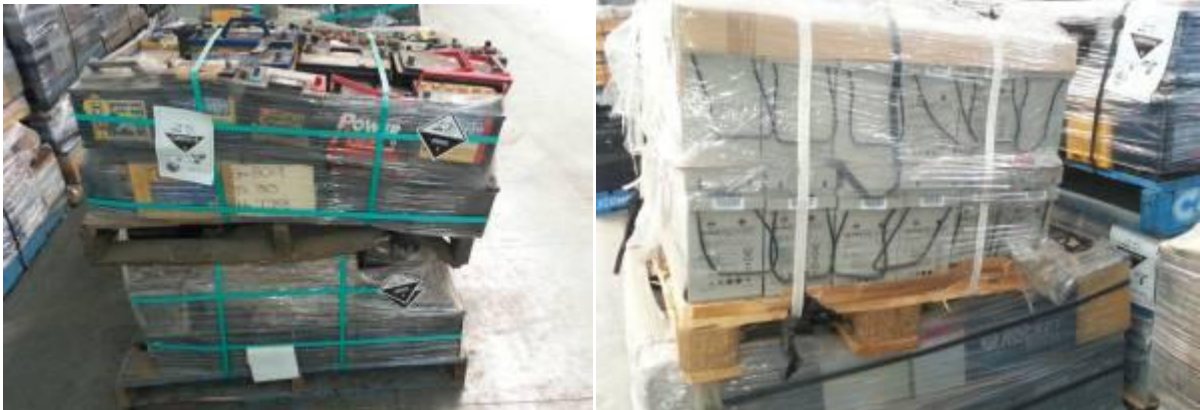
Fig. 41: Examples of bad packaging before transport, ABRI [26].
