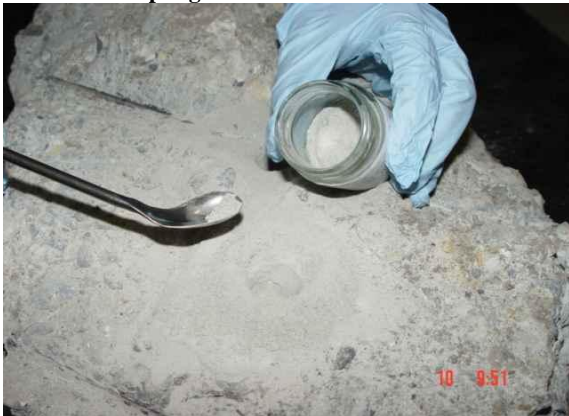
Picture 19: Sampling of concrete
