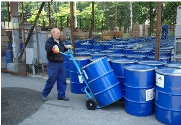
Picture 82: Safety Drum lift
