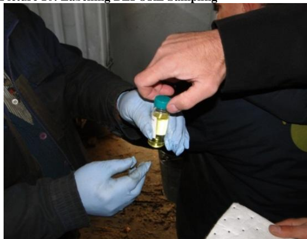
Picture 10: Labelling BEFORE Sampling
