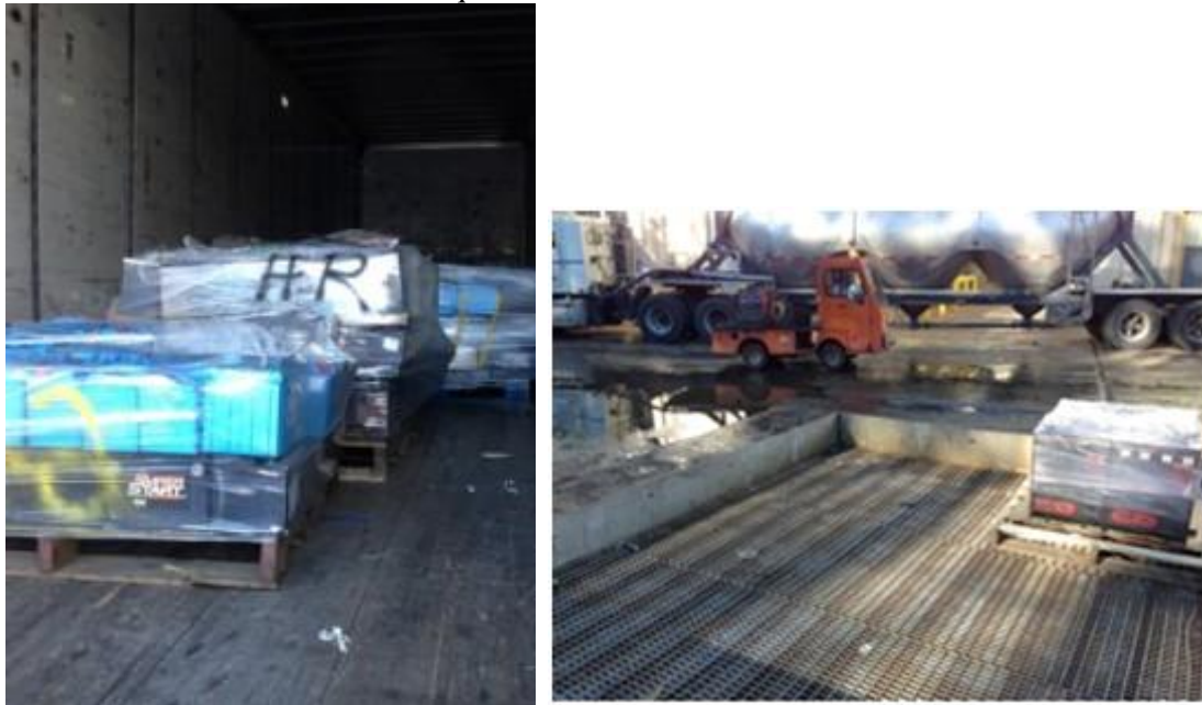
Fig. 12: Packaging of used lead batteries ready to transport – good example
