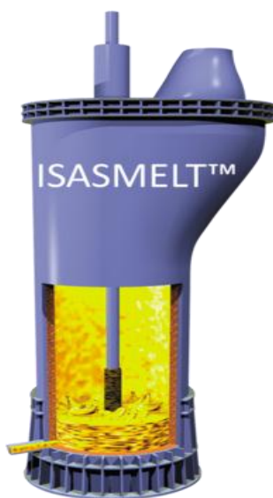
Fig. 26: Example of ISA Smelt furnace [31]
