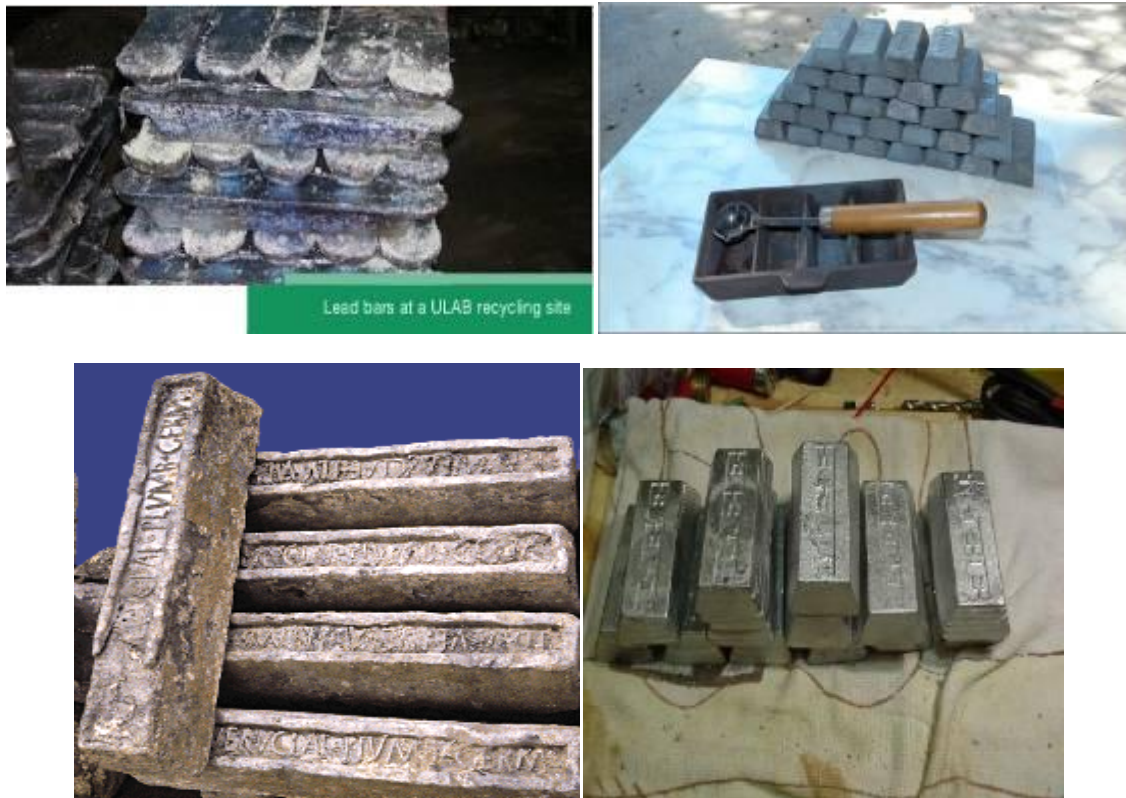
Fig. 32: Lead bars as the final product
