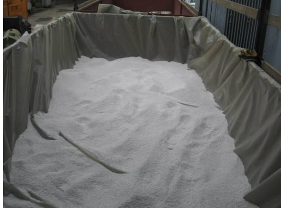
Picture 70: Covering the bottom with absorbent material
