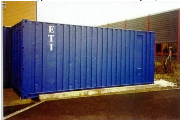
Picture 88: Typical 20' Box Container with trip tray
