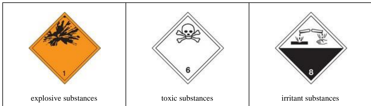
Fig. 11: Labelling of hazardous cargos according to ADR
