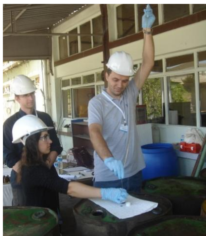
Picture 11: Sampling of oil drums
