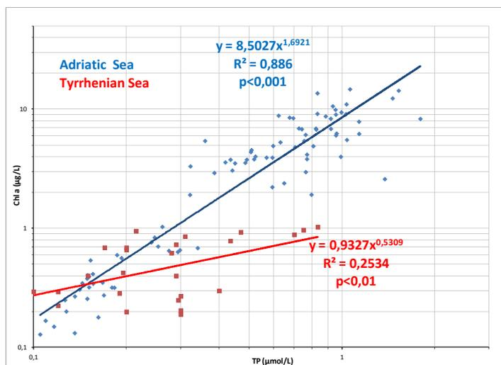
Figure 6.2: Chlorophyll *a* (Chl *a* geom. avg) vs. Total Phosphorus (TP geom. avg) concentrations (per sampling stations), in Adriatic and Tyrrhenian Seas. (From: Technical note on the classification criterion based on Chlorophyll *a*, as support to the MED GIG Milestone 5 report. (R. Precali, F.Giovanardi, J. Francé, S. Russo and C. Mazziotti)
