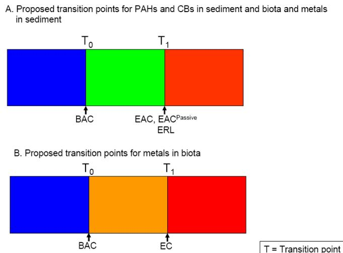
Figure 6.4: Illustration of the proposed traffic light system and the relevant transition point criteria for: A. PAHs and CBs in sediment and biota and metals in sediments, and B. metals in biota. The green/red boundary corresponds to the achievement of a statutory target (in WFD terms) or a policy objective (in OSPAR terms)
