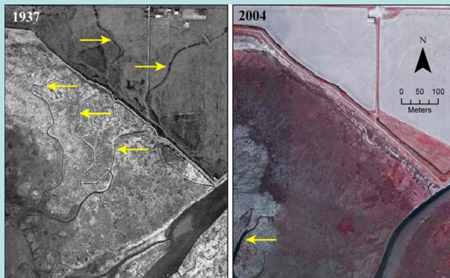
Fig. CS7: Remnant blind tidal channels in Skagit Delta marshes seaward (left-pointing arrows) and farmland landward (right-pointing arrows) of dikes constructed between 1870 and 1889. Blind tidal channels disappeared landward of dikes due to fill placement and rerouting drainage to ditches along property boundaries. Seaward of dikes they filled with resuspended bay sediments due to lost tidal prism. Only one shallow channel remains seaward of the dikes. The lower right corner of each photo shows a distributary, disconnected from the river by dikes in the 1950s. Much lower volumes of tide gate-mediated farm drainage, causing the remnant distributary to fill and narrow with resuspended bay sediments, replaced river discharge. The 1937 photo is courtesy of the Puget Sound River History Project. Both photos are at the same scale.
