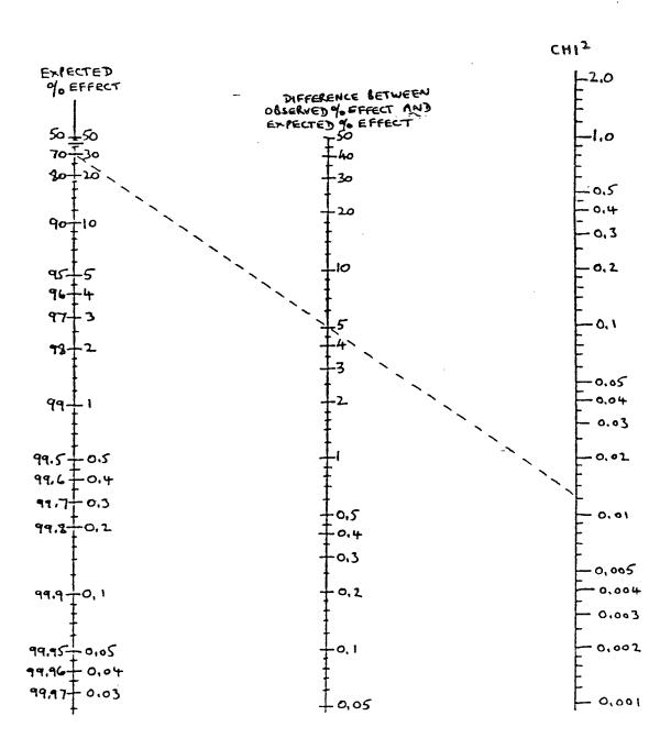
FIGURE 2. Nomograph for the determination of  ${\rm chi}^2$  (see 11.8). To use the nomograph, construct a straight line (or use a ruler) which connects the expected % effect value (on the left-hand axis) to the value of the difference between the observed and expected values (on the central scale). Project this line forward until it intersects the  ${\rm chi}^2$  axis on the right of the diagram. The  ${\rm chi}^2$  value is read from the intersection.
