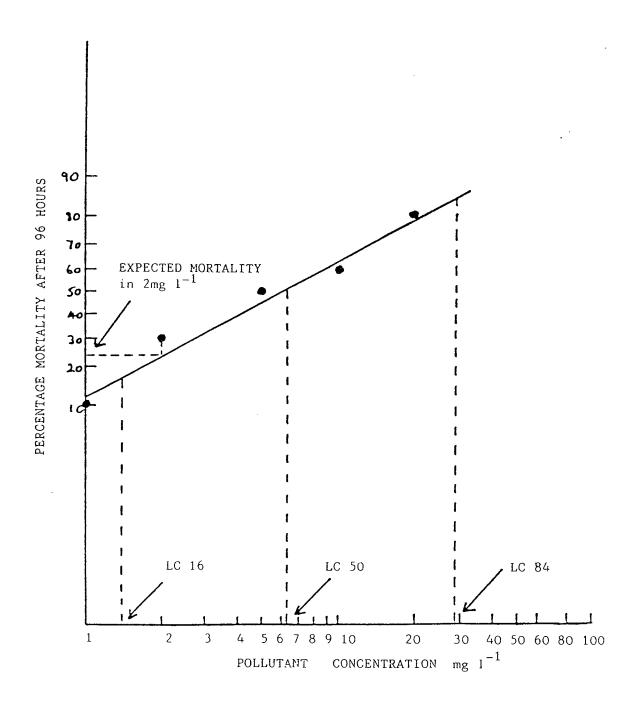
FIGURE 1: Estimation of the 96h LC50 value using the data given in Table 2. The diagram shows how values of LC16, LC84 are read off from the line and how the expected mortalities at each concentration are determined.
