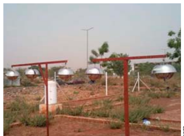
Passive air samplers in Mali
