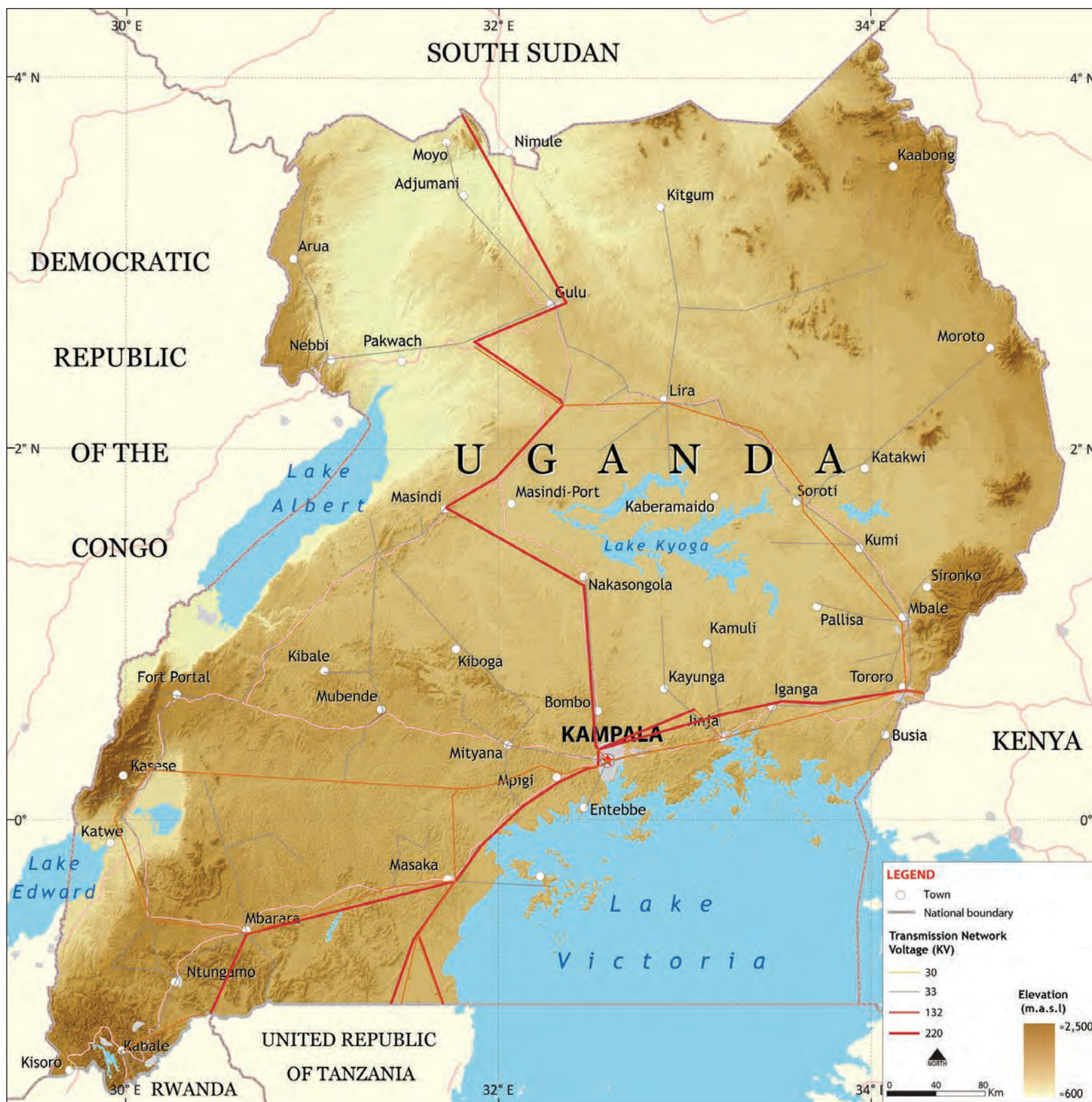
Figure 10.4: Existing power transmission grid coverage and generation site by 2014
