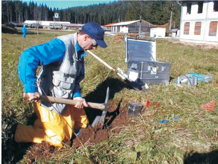
Soil profiles collected from Han Pijesak revealed limited dispersion of DU into the ground
