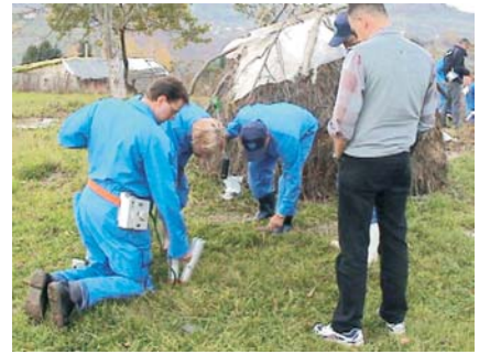
Gamma measurement of a cesium contamination spot
