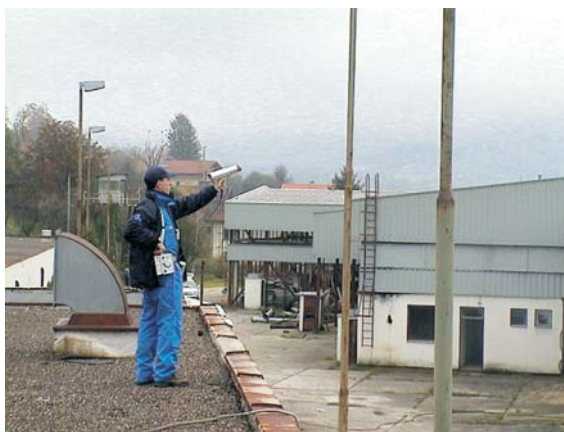
The radioactive source from lightning rods is another important issue to address
