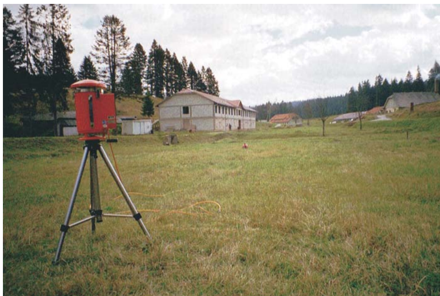
Air samplers were positioned throughout the site for an overall estimation on the presence of DU in air
