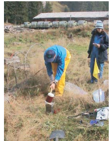
A large hammer is used to drive the soil profile plate into the ground
