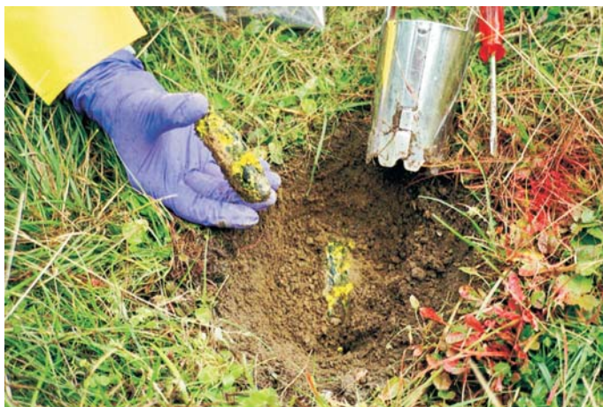
A heavily corroded penetrator is collected from the soil at Han Pijesak
