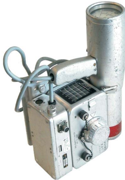
Saphymo-SRAT scintillometers measure gamma radiation
