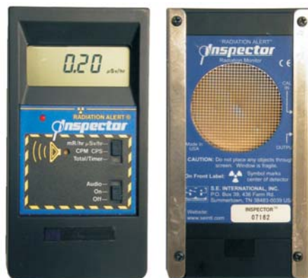
Inspectors can measure gamma, beta and alpha radiation
