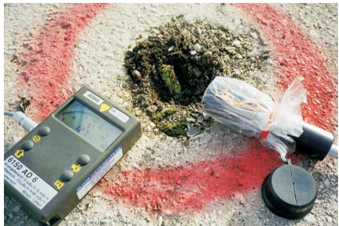
Beta radiation is measured from a penetrator fragment found in the concrete at Hadzici
