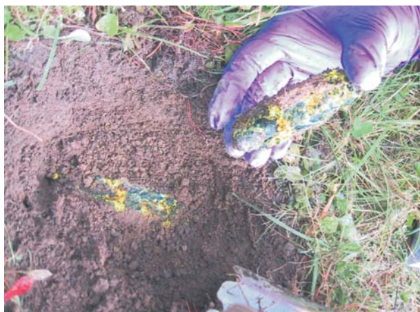
DU corrosion products are left behind in the soil
