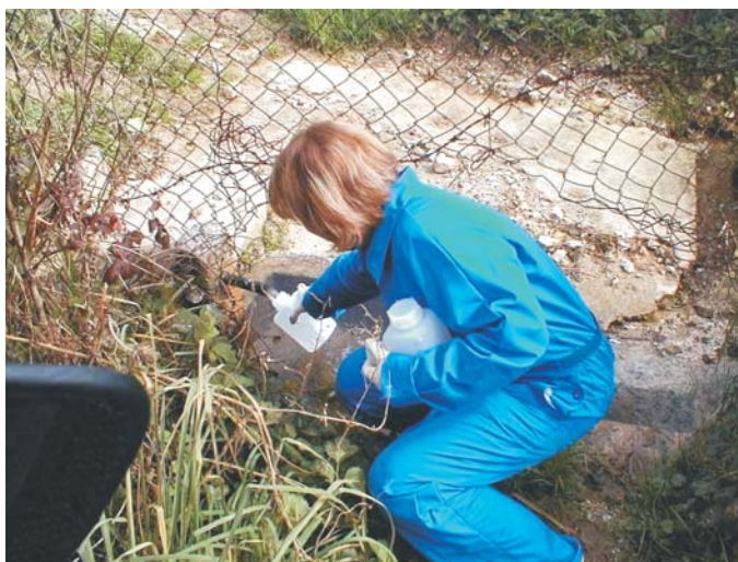
Collecting a water sample from a drainage well
