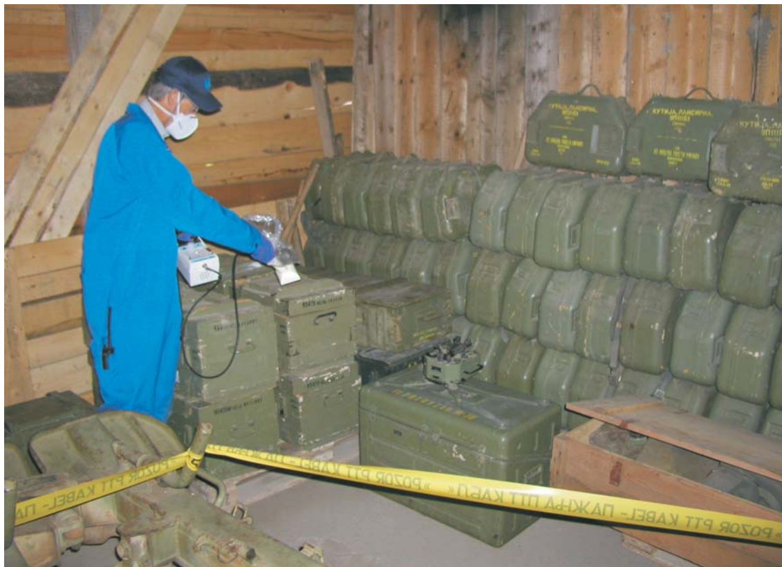
Both scratch and smear samples were collected inside the contaminated storage barn
