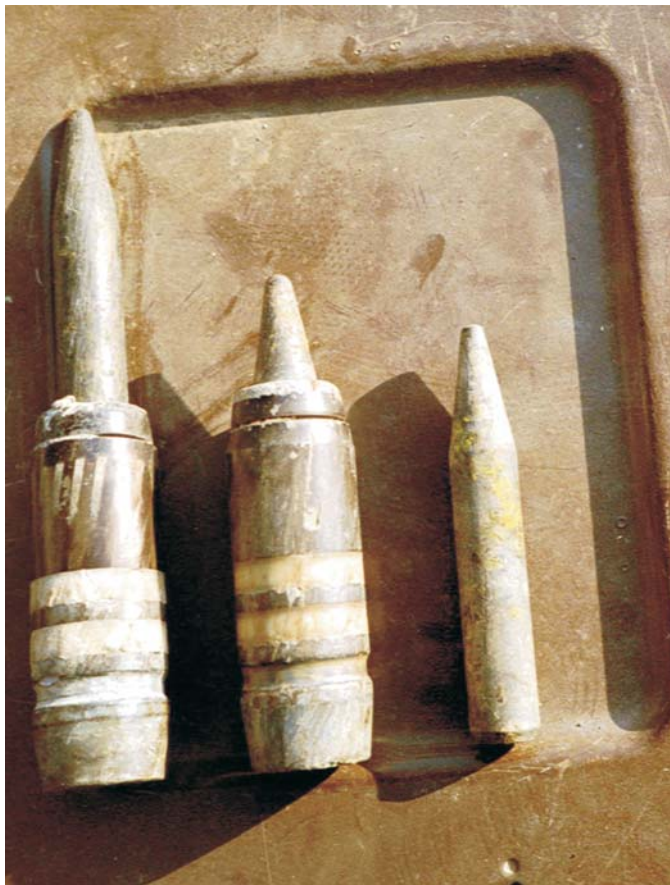
One penetrator (right) and two penetrators still fixed in their jackets. The left penetrator has partly moved from its position in the jacket.
