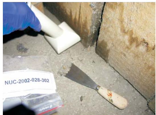
DU content of uranium in scratch samples exceeded 99%
