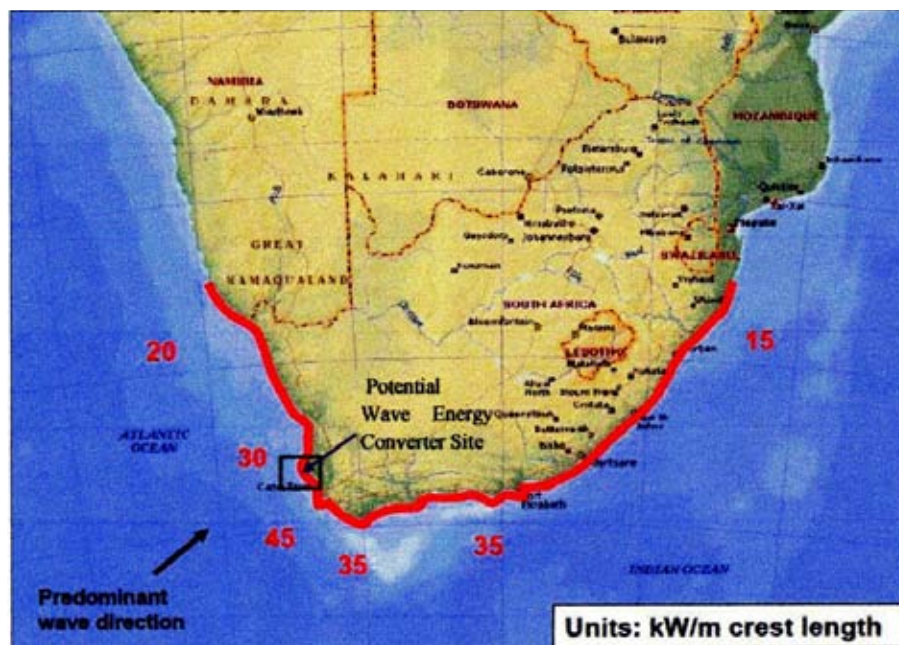
Figure 38: Varying off-shore annual average wave power levels along the southern African coast
