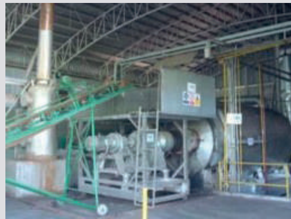
FIGURE 19: Pyrolysis plant processing plastic garbage into oil
