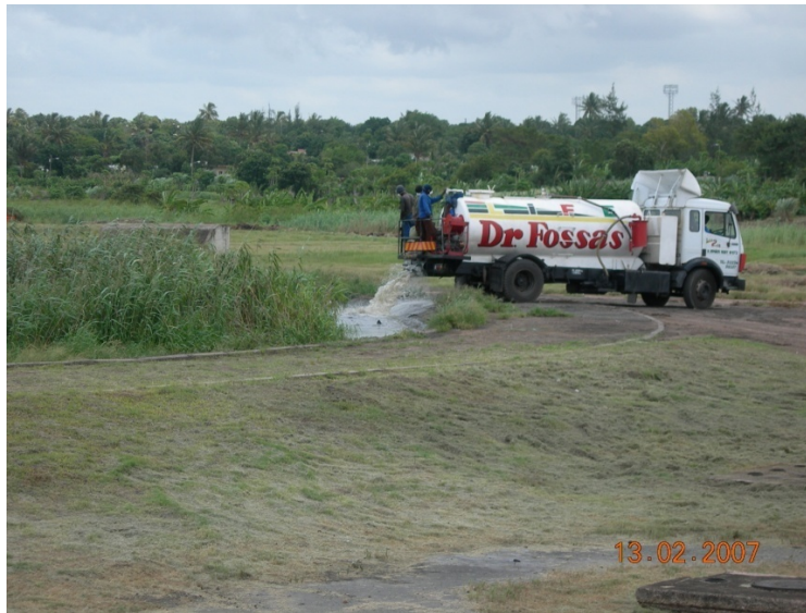
Figure 3.13 Cesspit emptier discharging wastewater containing sludge to waste stabilization ponds in Maputo
