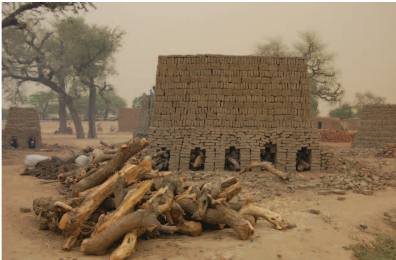
Traditional forms of brick making, like traditional stoves, are woefully energy inefficient.
