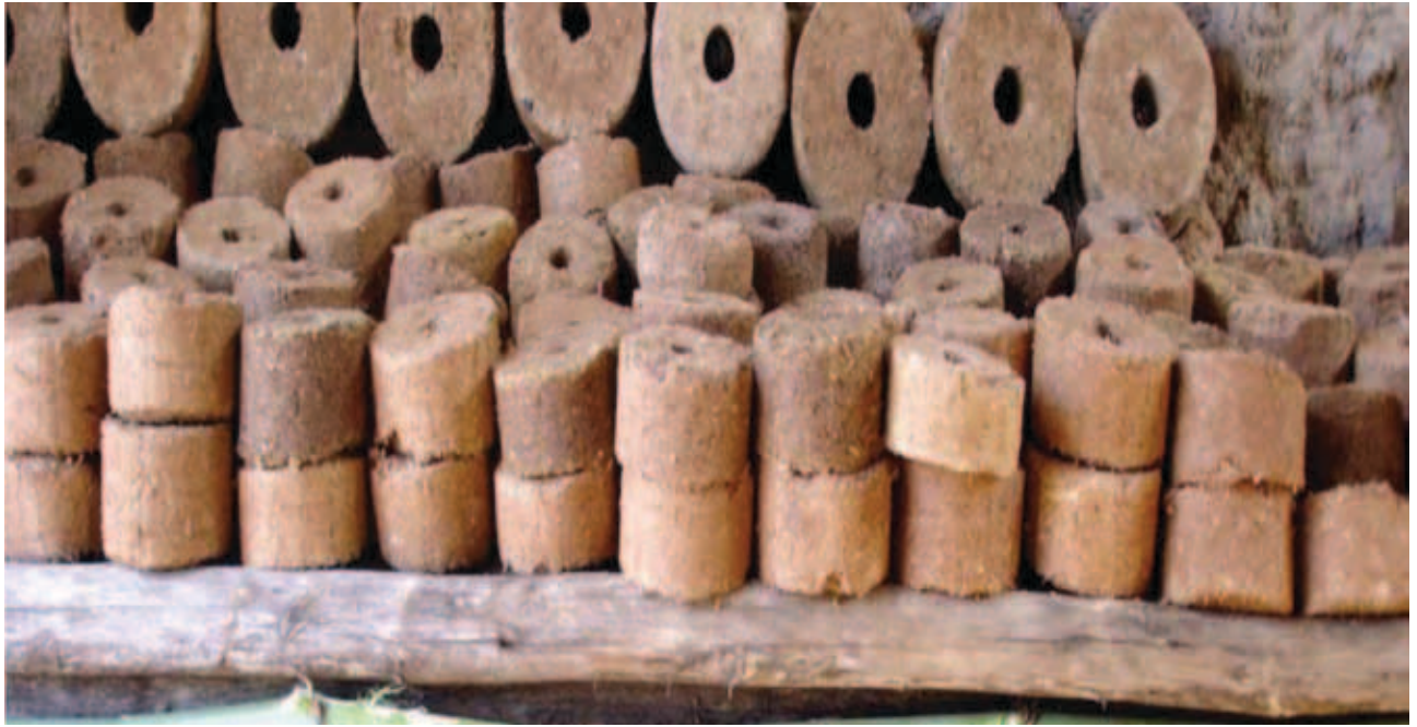
Figure 4.7. Biomass briquettes produced using the Legacy Press
