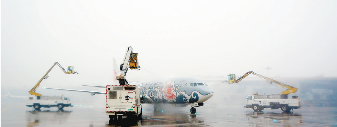
Fig. 3.8 Engine running deicing
