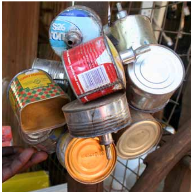
Kerosene wick lamps made from recycled cans
