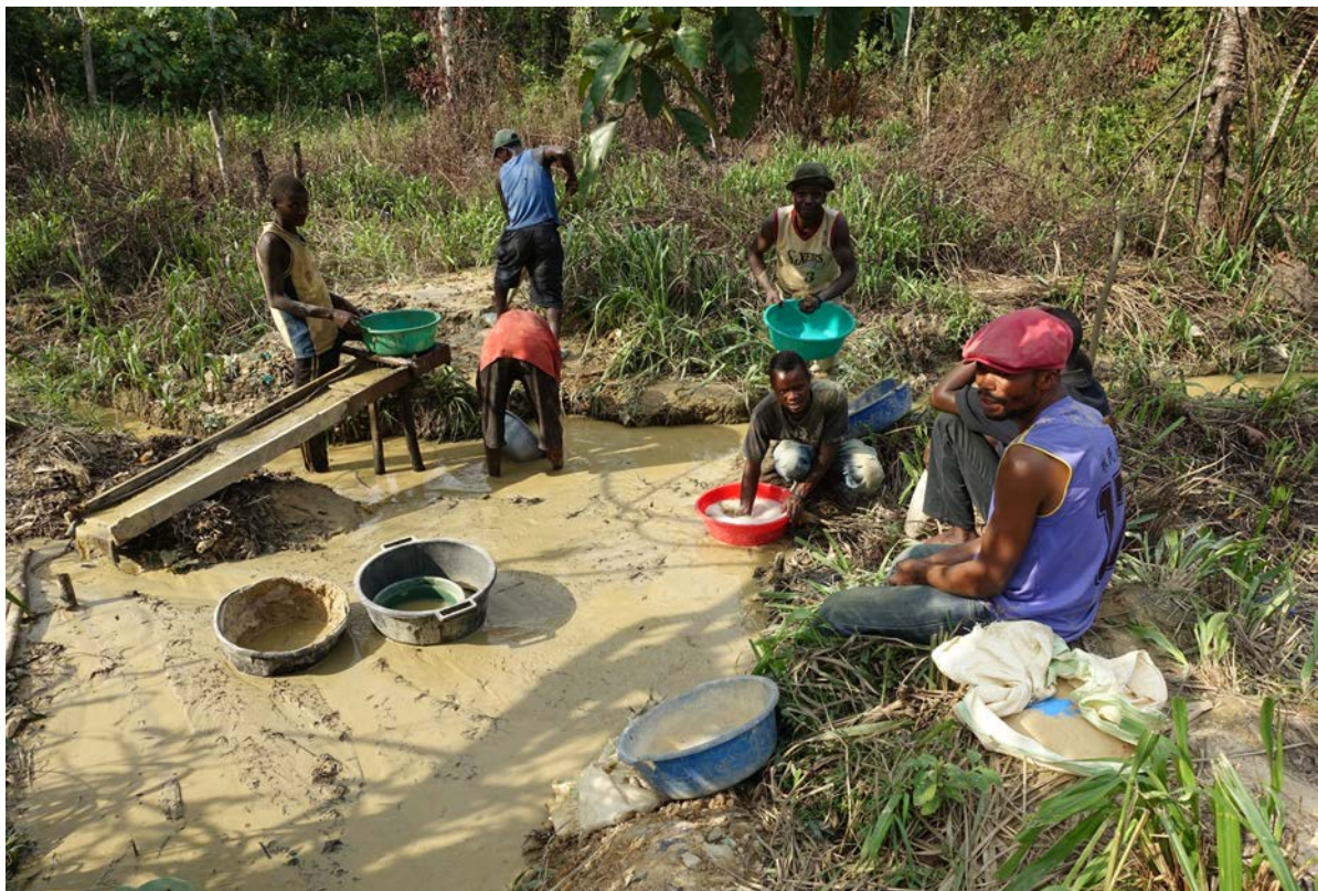
Photo 18: Continuous reprocessing of mine tailings. Note the lack of organized tailings storage, or effluent control
