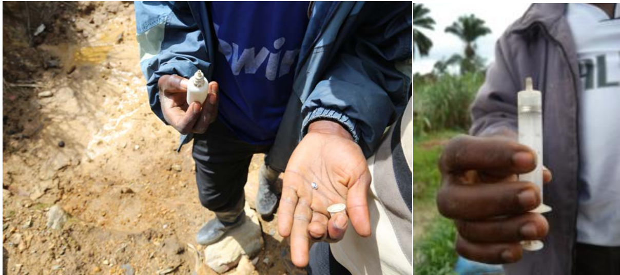
Photos 13 and 14: The PDG manages the mercury for the site, which is handed out for free to miners, and then collected in the same bottle or syringe after the excess is squeezed out of the amalgam
