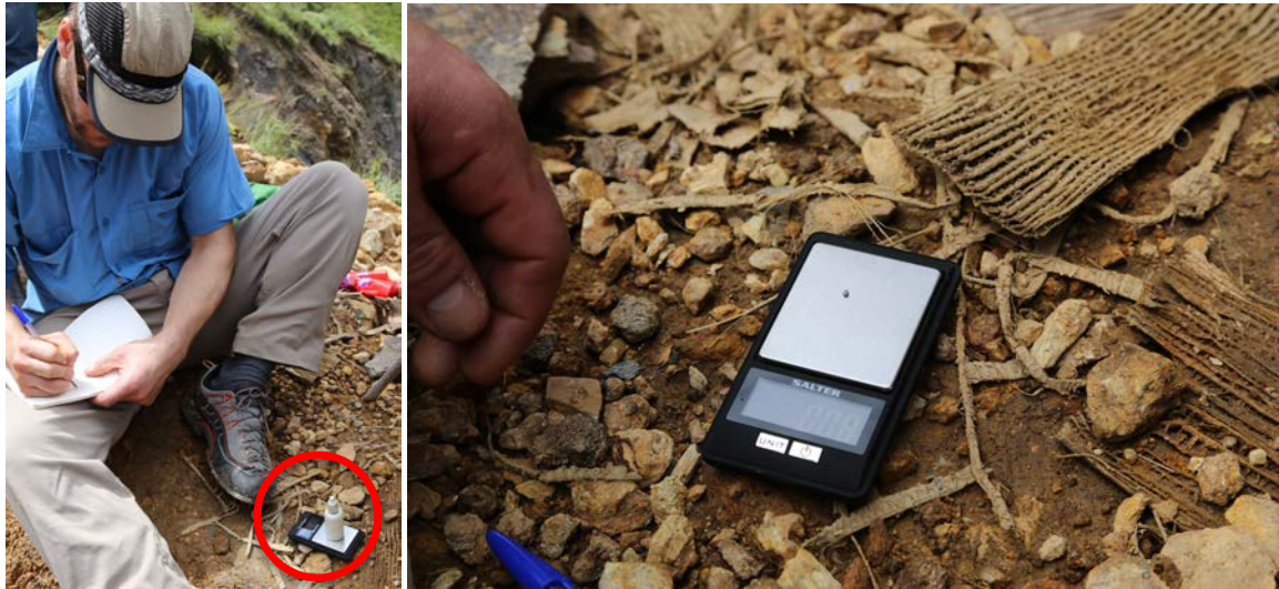
Photo 24 and 25: Mercury inventory using an electronic balance to measure ratio of mercury loss to gold produced
