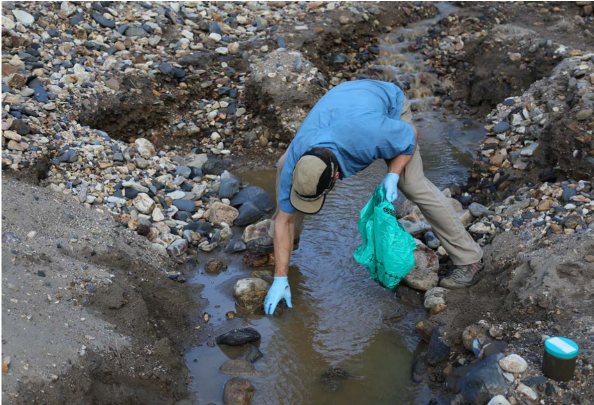
Photo 26: Sediment sample collection from the Luzinzi riverbed where alluvial mining is taking place
