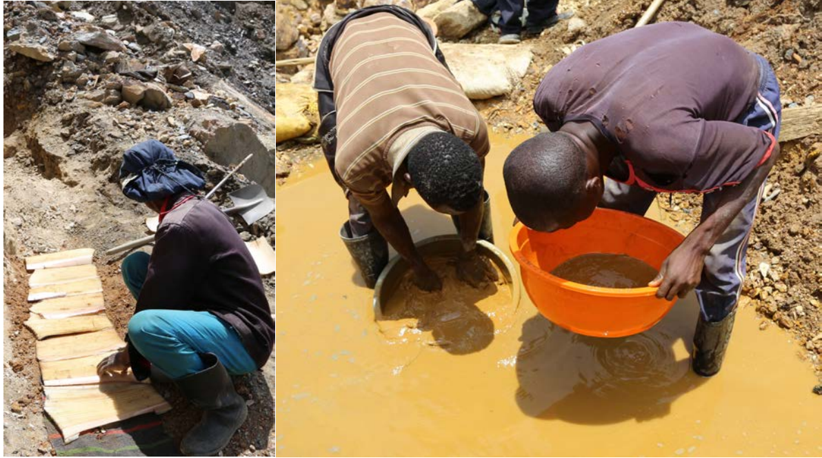
Photos 10 and 11: Banana bark makes an effective, if inefficient, gold concentrator (left). Proper carpets and a smooth, 10 sloped sluice bed would be more effective in capturing gold. Plastic wash basins make relatively poor gold concentrators, and proper gold pans would be more effective
