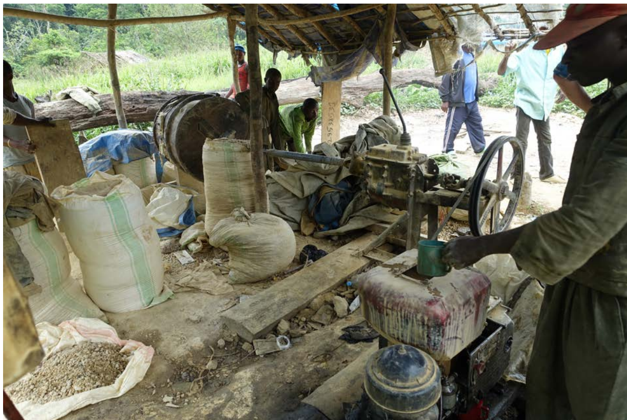
Photo 17: This old diesel motor must regularly be fed fresh oil to keep it running. The capacity of miners to improvise this rough but functional mill drive system, demonstrates their capacity to learn to operate best practices equipment
