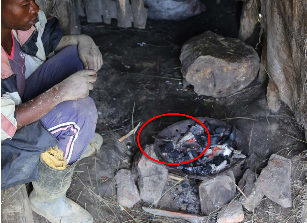
Photo 9: Open air burning of gold amalgam with a tablespoon on charcoal stove
