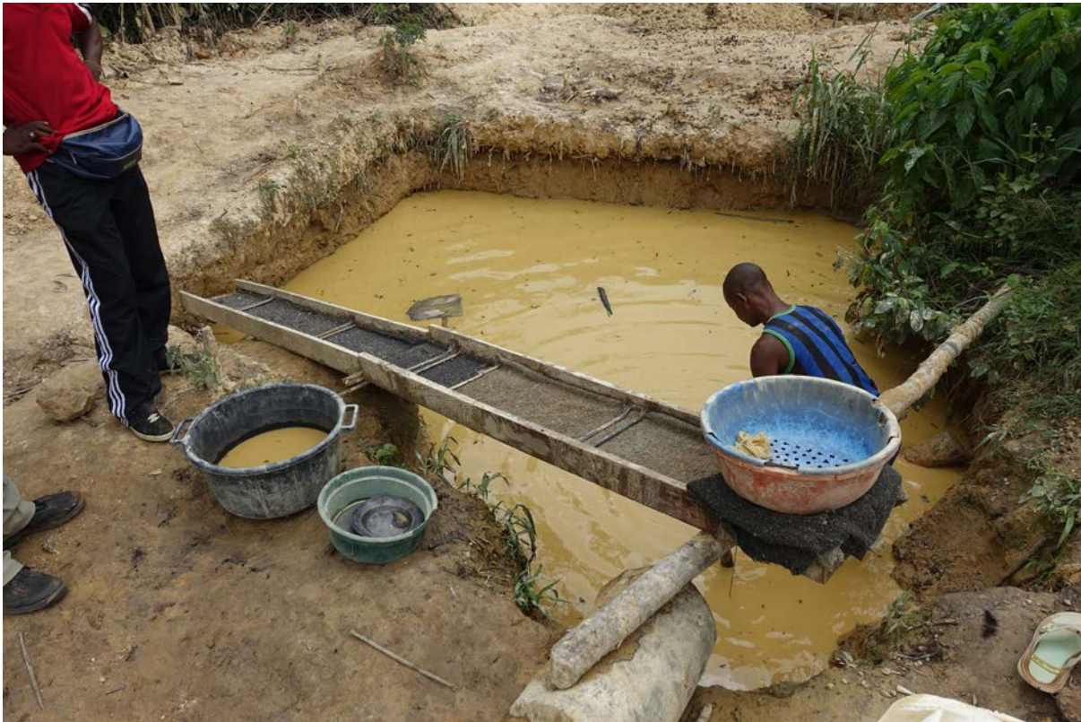
Photo 21: In Kafiawema the slope of this sluice could be optimized, and the two sluice sections should be arranged in L or Z configuration to force the flow to stop and restart (most gold is caught in the first metre of the sluice, making a turn gives more effective sluice length)
