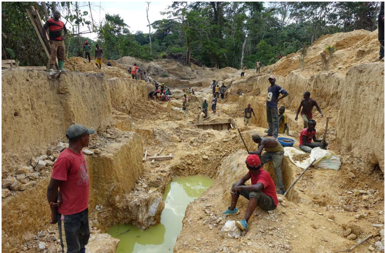
Photo 16: Open pit mines can only operate as long as the water is pumped out and pit walls are stabilized. This imposes limits on the depth of exploitation, and expands the area that must be cleared to sustain the same number of miners over time. Pits are dug with hand tools and water is removed with gas powered pumps
