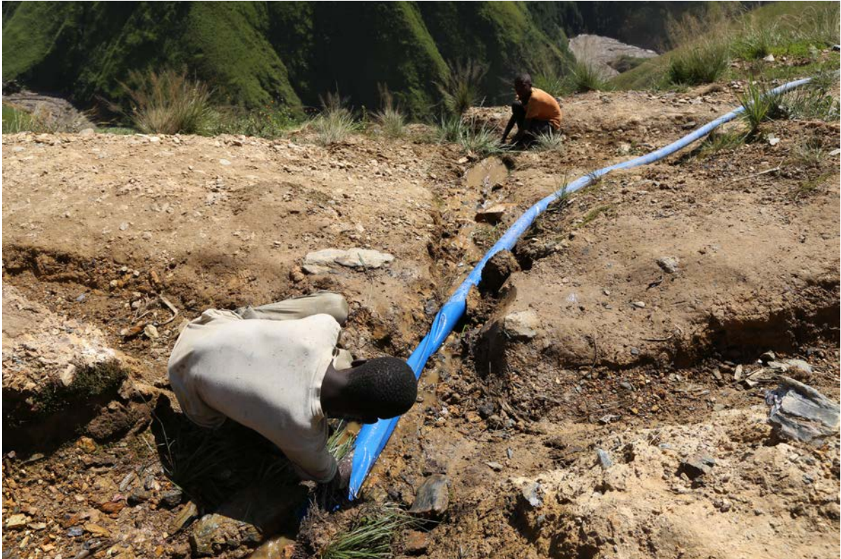
Photo 29: Hoses are sometimes used to deliver water for on-site process operations; a major challenge and cost for miners
