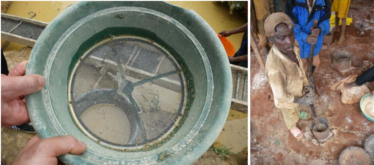
Photos 19 and 20: This (left) is probably an appropriate mesh size for the Kafiawema ore (approximately 1 mm), at least for the primary grind. Granulometric analyses would better indicate the optimal size. Mortar and pestle secondary milling (right)
