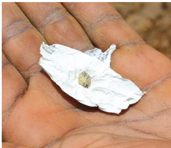
Photo 1: An amalgam of gold and mercury before burning
