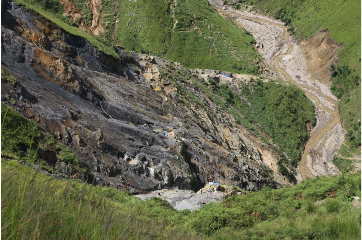
Photo 36: Steep slope mining in Butuzi poses serious risks of landslides which could dam the Luzinzi River below
