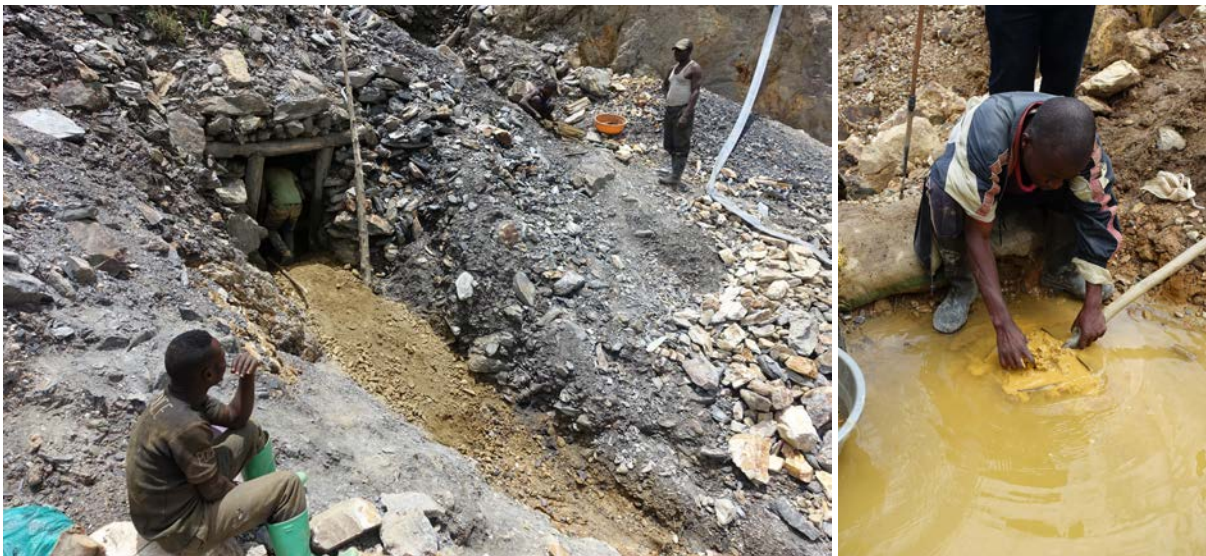
Photos 4 and 5: Rudimentary mine entrances and tunnels are sometimes buttressed by wooden beams, but these supports are few and tunnels are prone to collapse. Miners pan ore in shovels to test the gold content of ore
