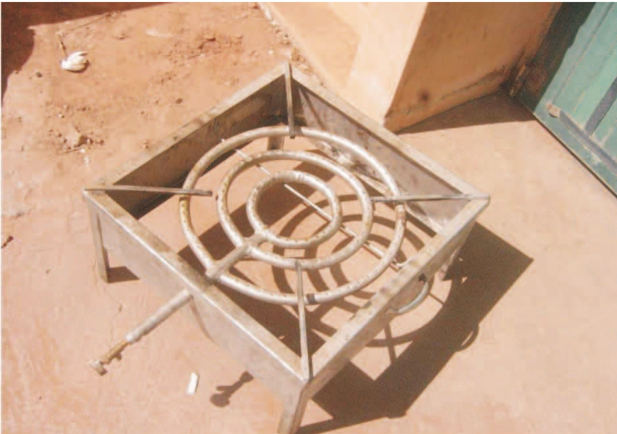
LPG stove for cooking Kisra developed by artisans in Khartoum. Despite attempts to adapt LPG appliances to cook local dishes, most households still prefer firewood and charcoal for cooking Asida and Kisra'
