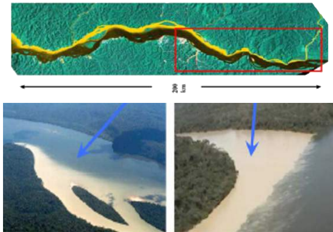
Figure 1-4. A false-colour Landsat satellite image and two aerial photos show the sedimentation caused by ASGM located on the Tapajos River, one of the largest tributaries of the Amazon River.
