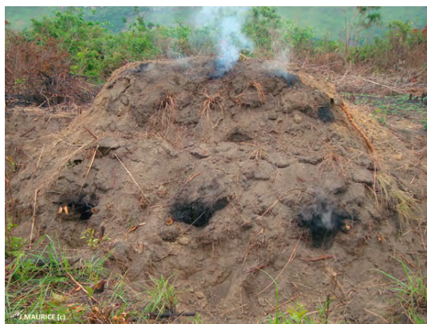
FIGURE 12: Improved traditional earth kilns in western Democratic Republic of Congo
