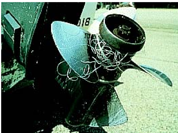
Figure 24. A boat that was wrapped by ropes around the propeller (Photo from the Ocean Conservancy).
