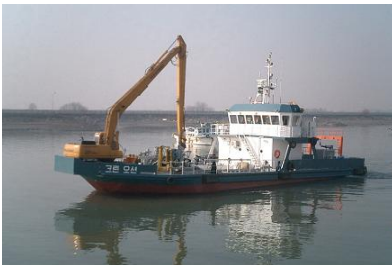
Figure 32. Specially designed vessel for marine litter collection, Ocean Clean .
