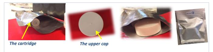
The cartridge must be kept inside the sachet throughout the experiment. It must keep this container pristine from mercury
