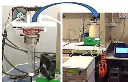
Figure 6. A prototype system for Hg-PAS thermal desorbing developed in CNR-IIA
