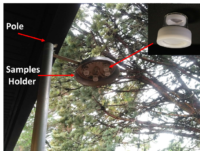
Figure 12. PAS setup used during the outside exposure comprising a shelter and N°. 8 housings for PASs.
