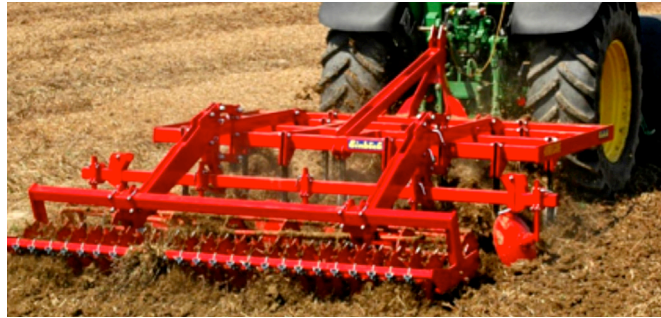
Figure 5: Shallow non-turning mechanical weed control
