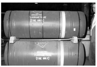
Photo 6-21 - Barrel of halon 1301 (bromotrifluoromethane).
