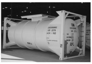
Photo 6-16 - ISO tanks allow for multimodal transport of large quantities of refrigerants.
