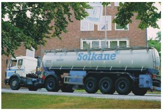
Photo 6-19 - Truck cistern used for transportation of large bulk quantities of HCFC-141b
