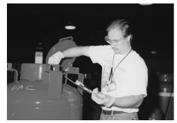
Photo 7-2. Conducting a temperature-pressure test.
