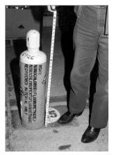
Photo 6-10 - "Recovered" R-502 (mixture of 49 per cent HCFC-22 and 51 per cent CFC-115) cylinder.
