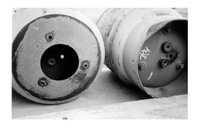
Photo 5-1. The access points to the main CFC-12 container become visible only after the double-layered container is cut open.
