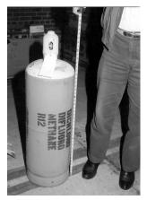
Photo 6-9 - Example of CFC-12 cylinder, dichlorodifluoromethane.
