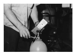
Photo 7-3. Example of a leak detector.
