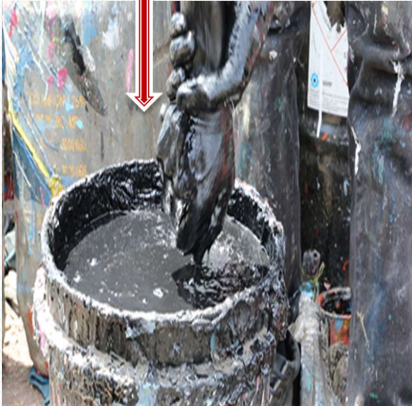
Formulation of paint using bare hands: Source (UNEP-Video footage-24 th – 26 th 2016- Kamukunji, Nairobi, Kenya)
