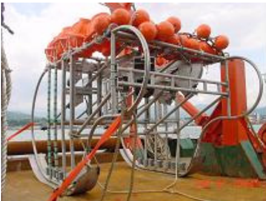
Fig. 5. Equipment to survey deposited fishing nets in 1,000m depth in NOWPAP Sea
