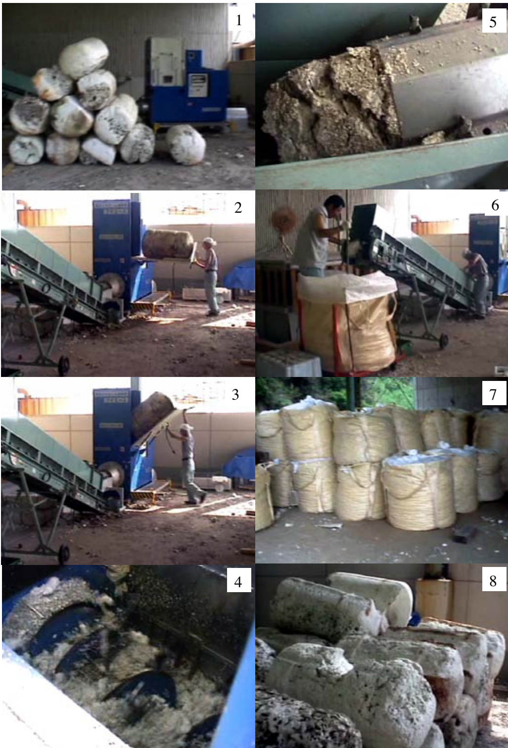
Photo 1. The process of the treatment of floats.
