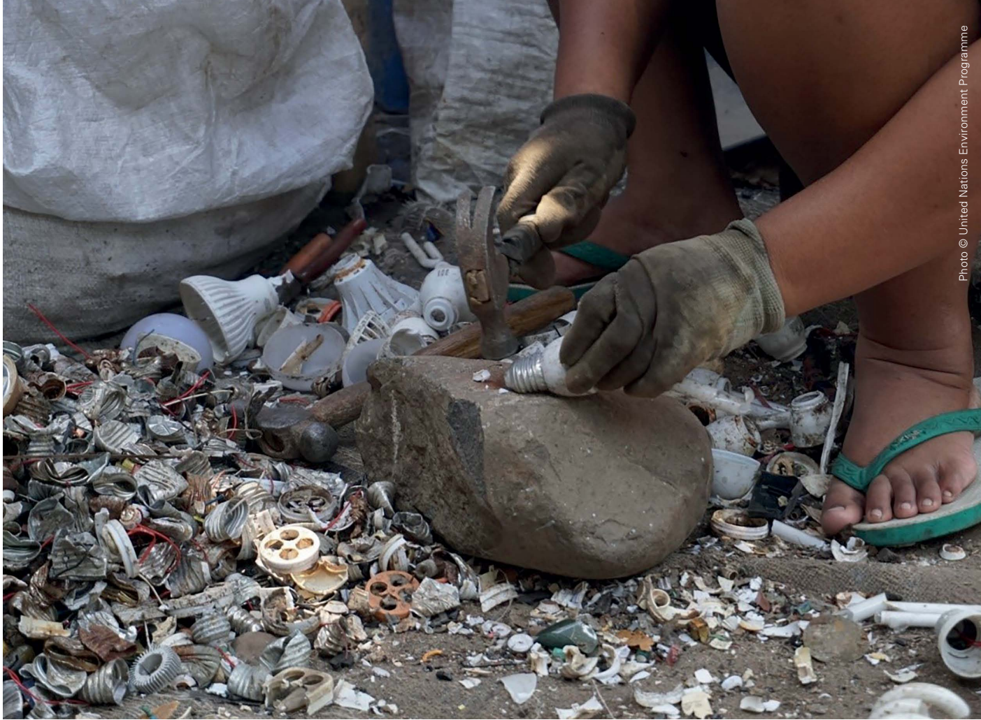
Crushing fluorescent lamps collected at the open dumping site to collect aluminium and copper as secondary resources
