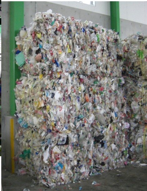
Waste plastics after compressed packing
