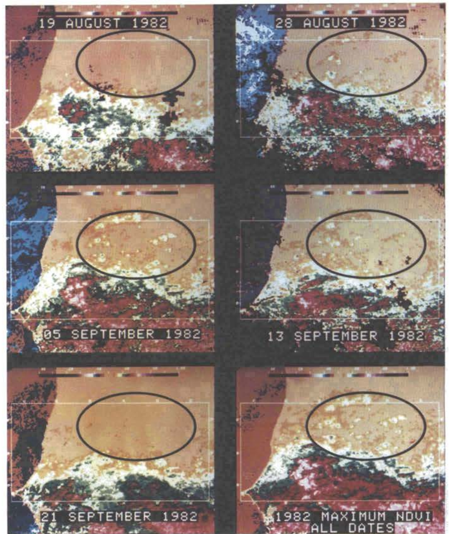
Figure 1: Time series development of green leaf biomass as indicated by NOAA-7 AVHRR data for southern Mauritania and northern Senegal in 1982. Note the complete cycle of green leaf biomass development in southern Mauritania occurred within an 18-day period. This graphically illustrates why AVHRR data are the only satellite data source capable of detecting these transient patches of green biomass development because temporal resolution is crucial while spatial resolution is not (from Tucker et al. 1985b).
