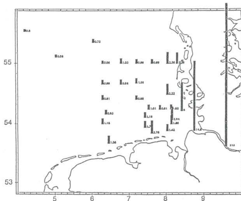
Figure 1: THC distribution in the German Bight, Jan. 1990 in \mu\text{g/l} (Source:THEOBALD et al., 1995).
