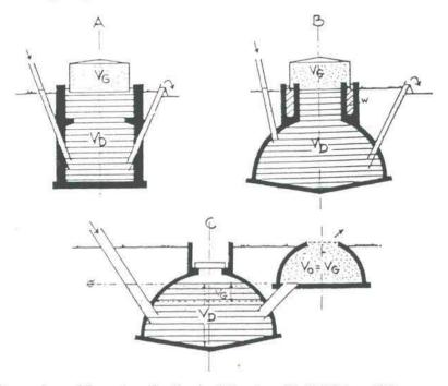
Figure 16: Comparison of Sasse-type family-sized digester with KVIC type (35)
