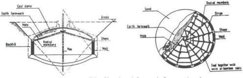
Umbrella-shaped formwork for casting dome
