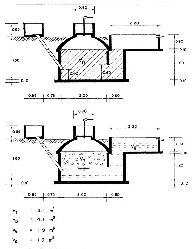
Figure 12: Fixed-dome digester designed by the National Energy Administration (NEA) (adapted from 5)
