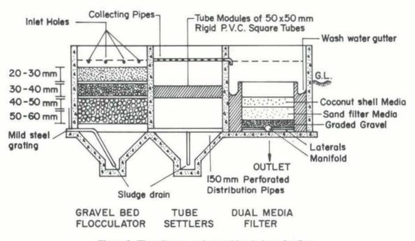
Figure 6. Flow diagram and ground-level view of upflowdownflow plant in Varangaon (Schulz & Okun, 1984)
