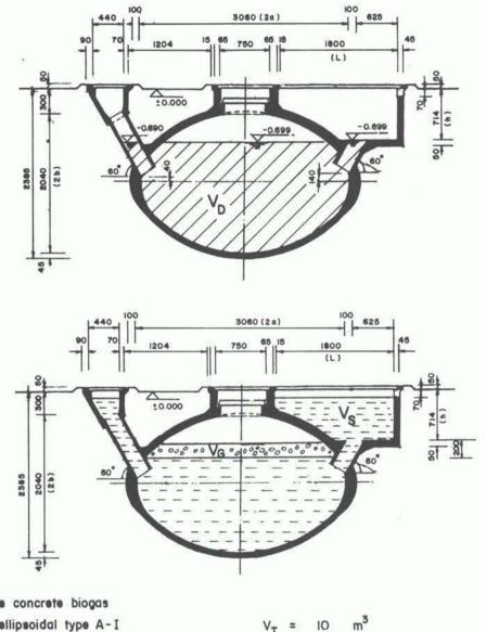
m<sup>3</sup> 10 = 9.0 m<sup>3</sup> = 1.1 m<sup>3</sup> VG = I.I m<sup>3</sup> (0.25 m<sup>3</sup> gas/m<sup>3</sup> d) Vs =
