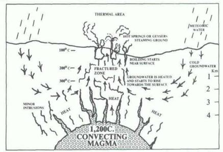
Figure 1. Model of a geothermal system showing the convection mechanism by which rising hot water is replenished by precipitation (the cycle can span hundreds of years).
