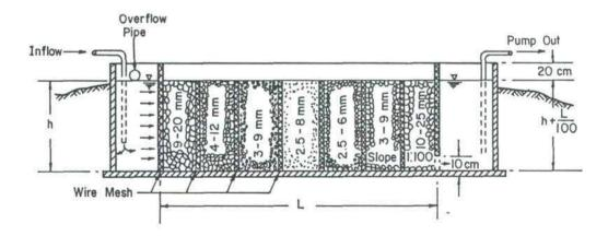
Figure 2 Horizontal-flow coarse-media filter
