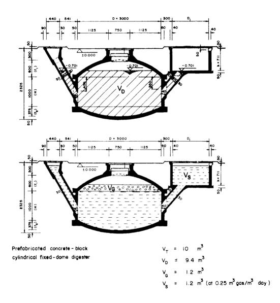
Figure 1: Prefabricated concrete-block cylindrical fixed-dome digester (adapted from 14)
