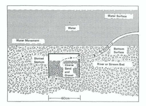
Figure 5. The SWS water filtration system (Cansdale, 1979)
