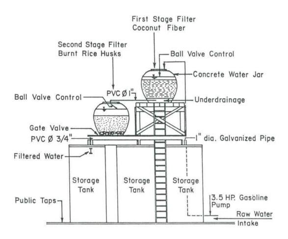
Figure 4. Two-stage filtration unit constructed at Ban Som, Korat, Thailand
