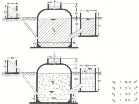
Figure II: Fixed-dome digester designed by the Sanitation Division (adapted from 20)
