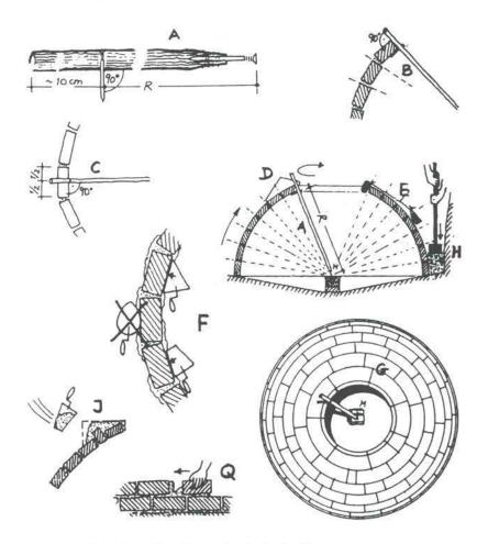
Construction of a spherical shell from masonry. Figure 18: Normal method of construction of bottom and shell (adapted from 35).
