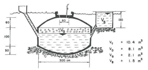
Figure 13: Fixed-dome digester designed by Department of Agricultural Extension (DOAE) (adapted from 20)
