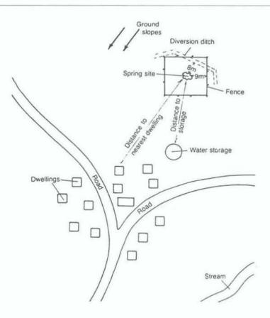
collection of spring water flowing from a single opening on level ground. To determine which design to use dig out around the area until an impervious layer is reached, locate the source of the spring flow and design to fit the situation.
