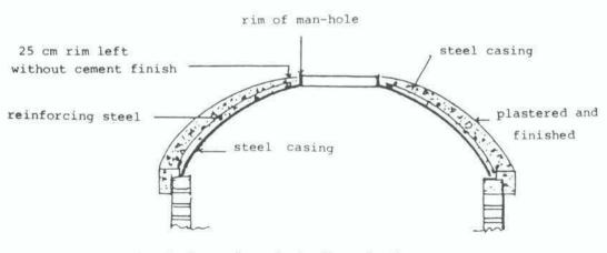
Vertical section of the dome showing details of concrete casting
