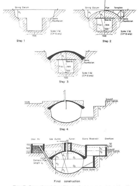
Figure 10: Construction technique of Nepalese fixed-dome design, (adapted from 19).
