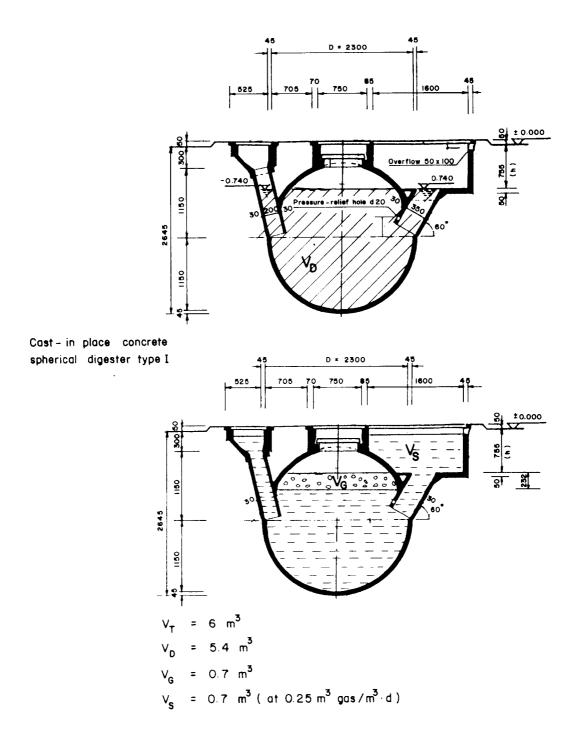
Figure 2: Cast-in-place spherical digester Type I (adapted from 14)
