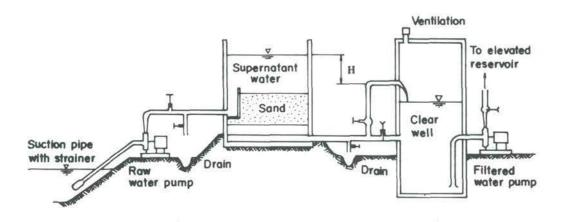
Figure 1. Simplified operation of slow sand filter (Huisman, 1978)
