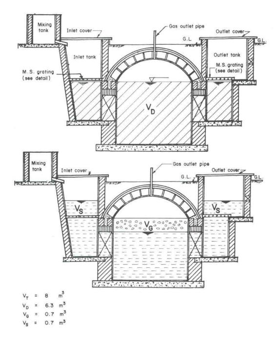
Figure 8: Design of a Janata plant of 8m<sup>3</sup> total digester volume adapted from (25)
