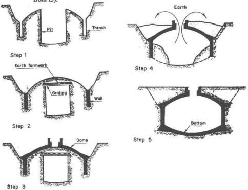
Figure 5: Construction technique for concrete cast-in-place digester (adapted from 15)
